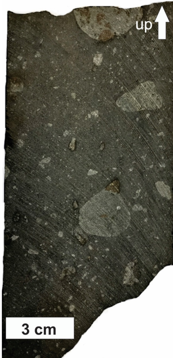
Figure 16: Oriented drill-core sample DD1012_16 at 74 m depth from Kakula of the middle diamictite from drill-hole DKMC_DD1012, approximately 250 m above the ore-zone. The diamictite is generally textureless with clasts of various sizes in fine-grained matrix. In hand sample, the middle diamictite appears to have characteristics similar to diamictite of the basal diamictite for clast composition, sizes, and percentages. The middle diamictite is generally green-grey to grey like the basal diamictite outside of hematite-rich zones.
