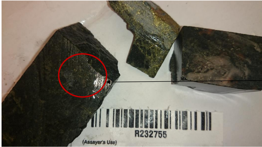
Transect 3: Sample R232755 of mineralization along a 220 trending sulfide vein. Note the disseminated sulfides within the chloritized matrix
