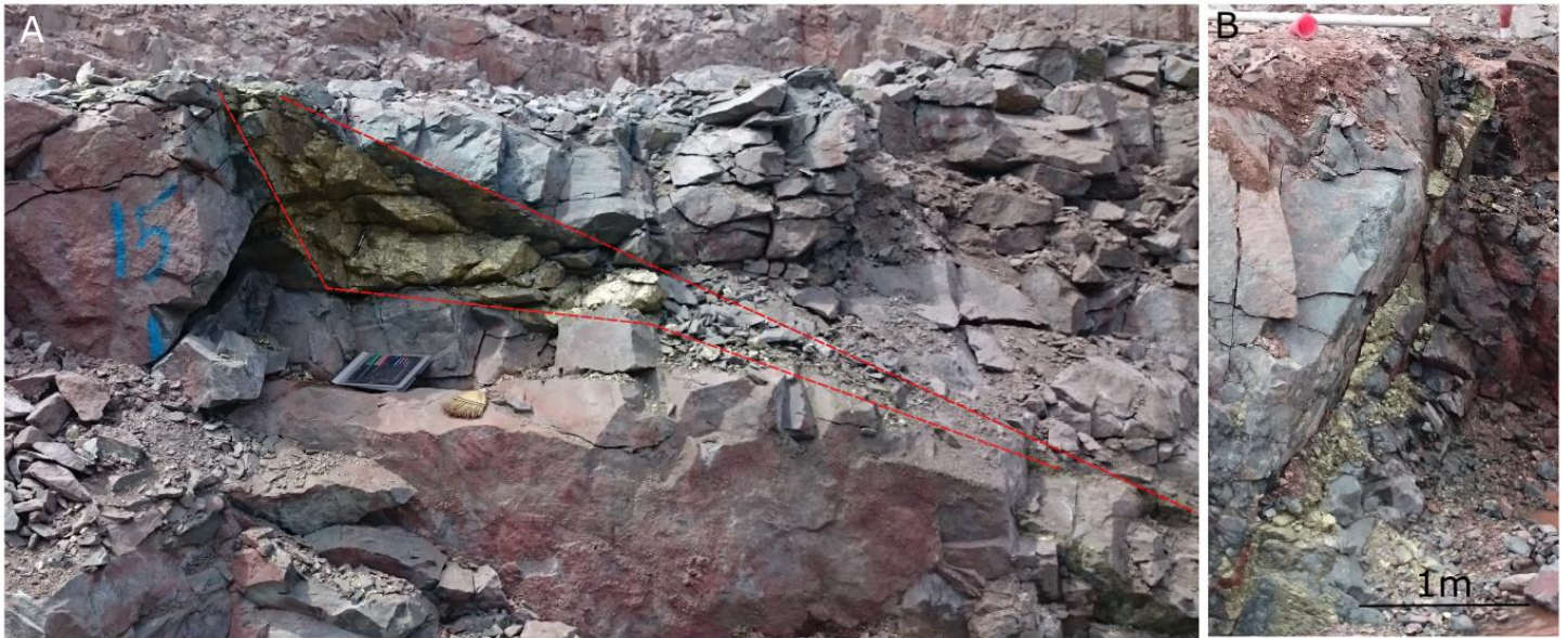
Pinch and swell pattern of sulfide veins. A) Demonstrates pinching along dip from 50cm to <5cm. B) Demonstrates pinching in vein along strike.
