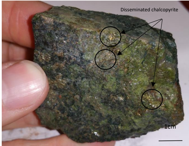
Low sulfide: Sample R232643 showing disseminated chalcopyrite within chlorite overprinting epidote
