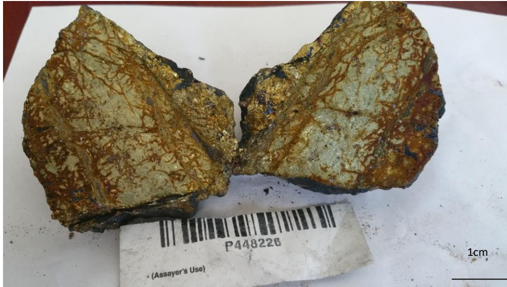
Transect 5: Sample P448226 of semi-massive sulfide bounding a core of highly altered Sudbury breccia
