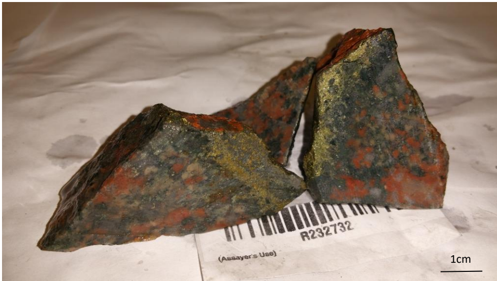
Transect 10: Sample R232732 of semi-massive sulfide cutting thermally altered pegmatitic granite
