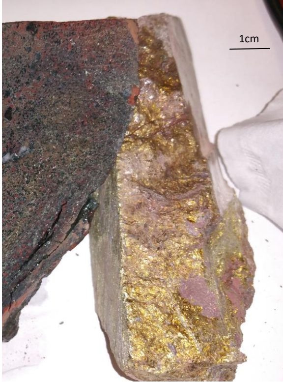
Transect 9: Sample R232663 showing the mix of massive chalcopyrite and altered country rock
