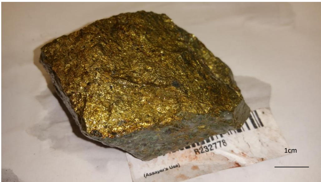
Vein set 08: Sample R232778 of massive sulfide.
