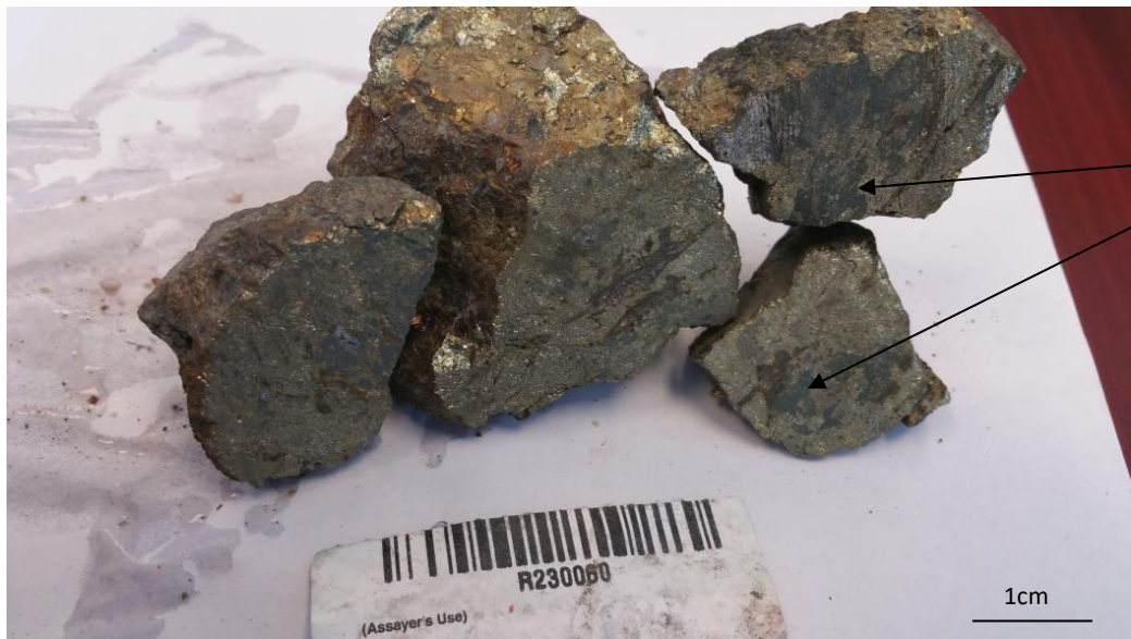
Transect 4: Sample R230060 of massive chalcopyrite. Note how chlorite replaces clasts within the sulfide
