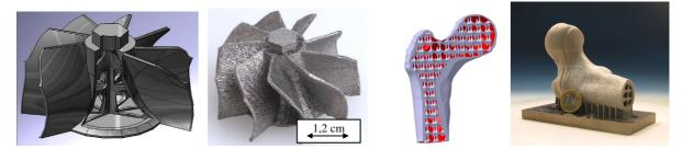
Fig. 5: CAD model and Laser Melting part out of Inconel 718 (left), CAD model and implant with internal structure (right)
