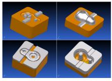
Fig. 14: Die casting (left) and injection molding (right) inserts
