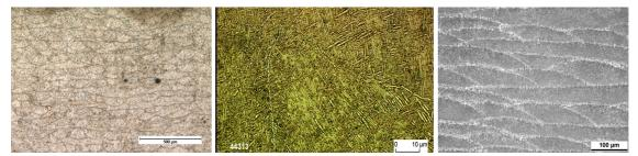
Fig. 1: Cross sections of Laser Melting parts, Tool Steel H13 (left), TiAl6V4 (middle), AlSi10Mg (right)
