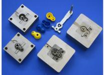
Fig. 15: CMB-made injection molding (left) and die casting (right) inserts together with molded parts
