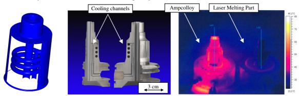
Fig. 3: CAD model (left), manufactured Laser Melting part (tool steel H13, manufacturing time 18 hours, middle) and thermographic image of Ampcolloy and Laser Melting part (right) (in cooperation with Braun GmbH)
