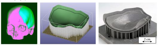
Fig. 4: CAD construction using CT-data (left), data preparation for Laser Melting (middle) and actual Laser Melting part out of Titanium GdII (right)
