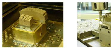
Fig. 8: Positioning system for laser sintering (left), milling and die spotting (right)
