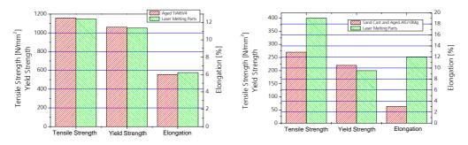
Fig. 2: Mechanical properties of TiAl6V4 (left) [3] and AlSi10Mg (right) [4] parts
