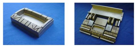
Fig. 9: Laser sintered module (left) and modules of reference tool (right)
