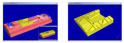
Fig. 7: Automatic calculation of sinter geometry and STL-data of the mold insert
