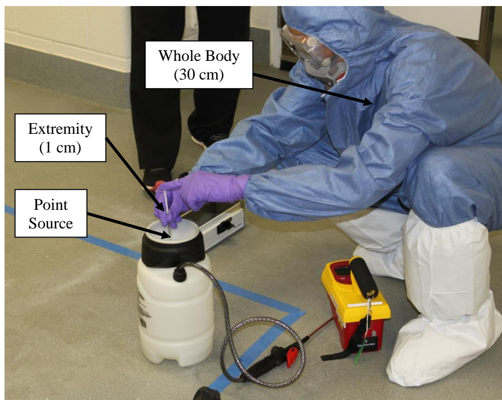
Figure 2.5 External Exposure Description During Mixing (Photo Taken During Dry-Run).
