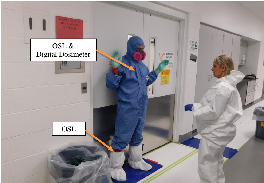
Figure 2.22 Dosimeters Worn by Exercise Participant used for Validation.
