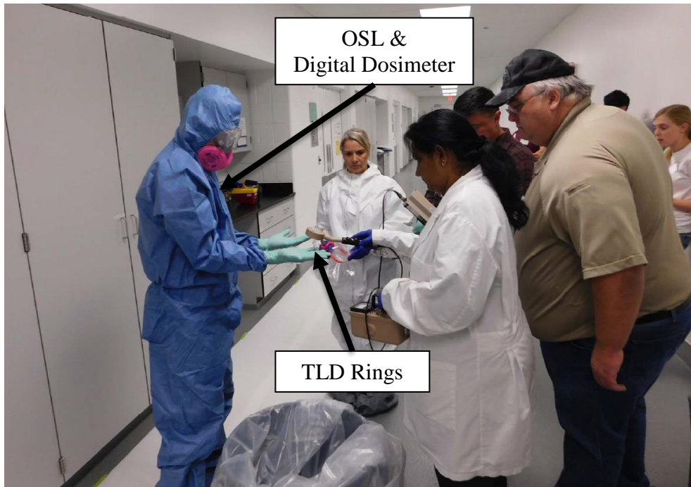
Figure 2.21 Dosimeters worn by Radiation Worker used for Validation.
