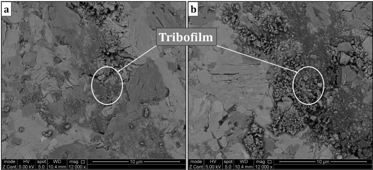
**Fig. 13a.** SEM micrographs of the pre-transition phase of the Maxthal 312/Al<sub>2</sub>O<sub>3</sub> sliding surface.
