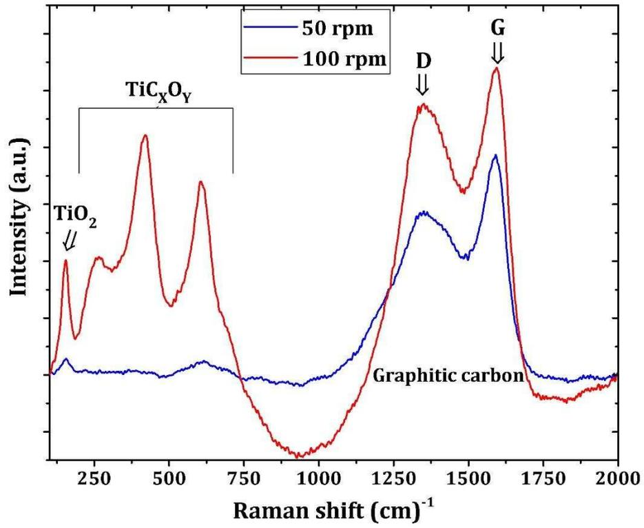
**Fig. 10.** Raman spectra acquired inside the wear track of the Maxthal 312-TiC/Al<sub>2</sub>O<sub>3</sub> tribocouples.
