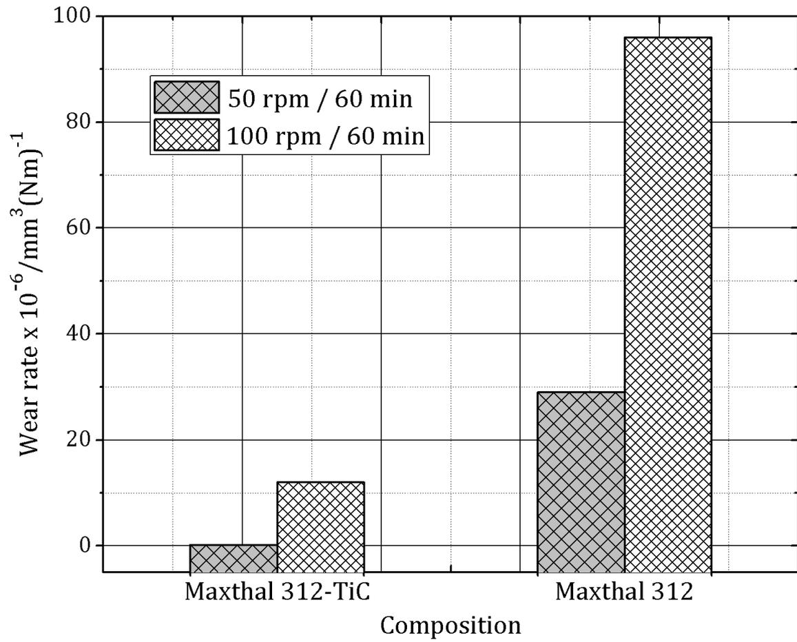
**Fig. 6.** The wear rates of the SPSed bulk samples upon sliding against Al<sub>2</sub>O<sub>3</sub> ceramic ball at RT.
