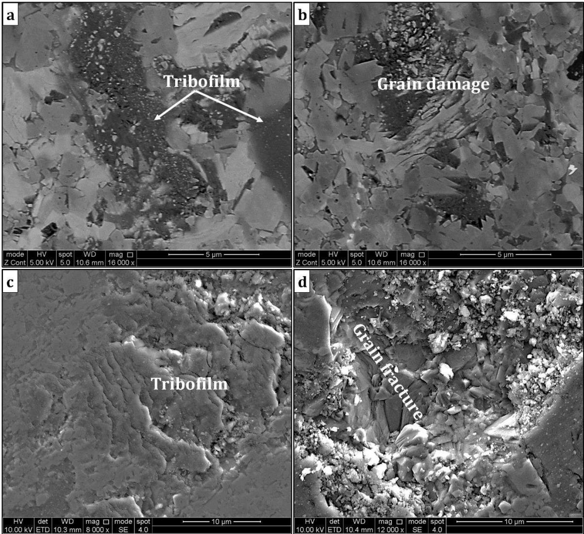
**Fig. 15.** SEM micrographs of the sliding surface of the Maxthal 312-TiC/Al<sub>2</sub>O<sub>3</sub> for the contact condition 50 rpm for 60 min (a-b), and 100 rpm for 60 min (c-d).
