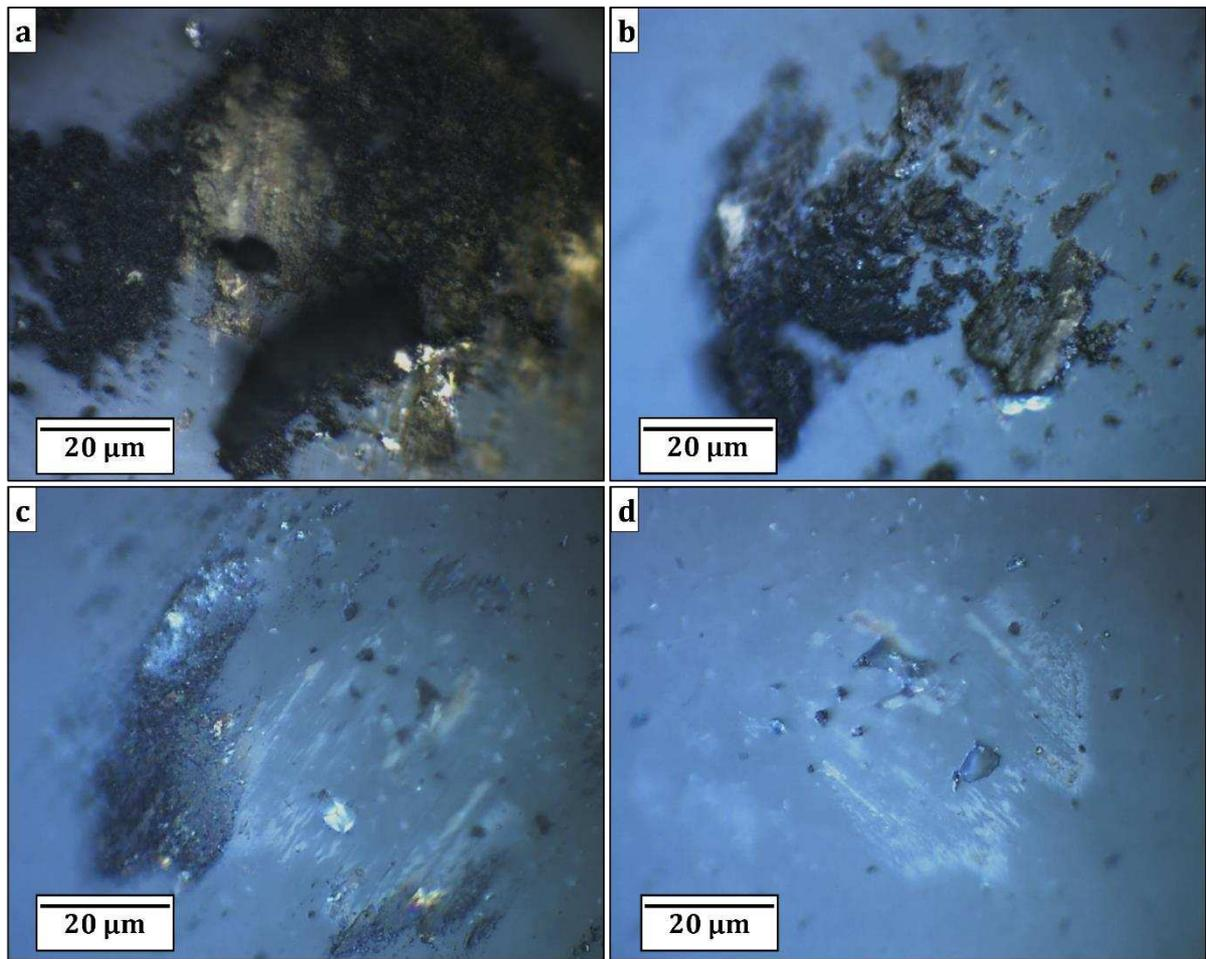
**Fig. 11.** Optical images of the  $\text{Al}_2\text{O}_3$  ball surface after unlubricated sliding against the Maxthal 312 disc ((a) before cleaning and (b) after cleaning) and Maxthal 312-TiC disc ((c) before cleaning and (d) after cleaning) discs for the contact condition 50 rpm for 60 min.
