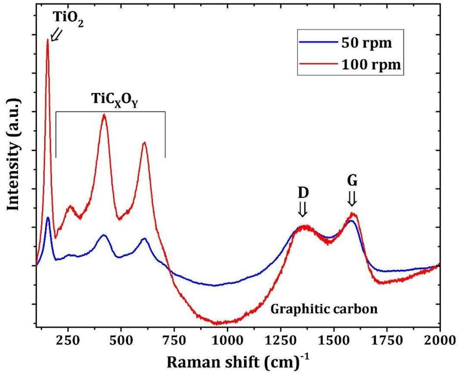
**Fig. 9.** Raman spectra acquired inside the wear track of the Maxthal 312/Al<sub>2</sub>O<sub>3</sub> tribocouples.
