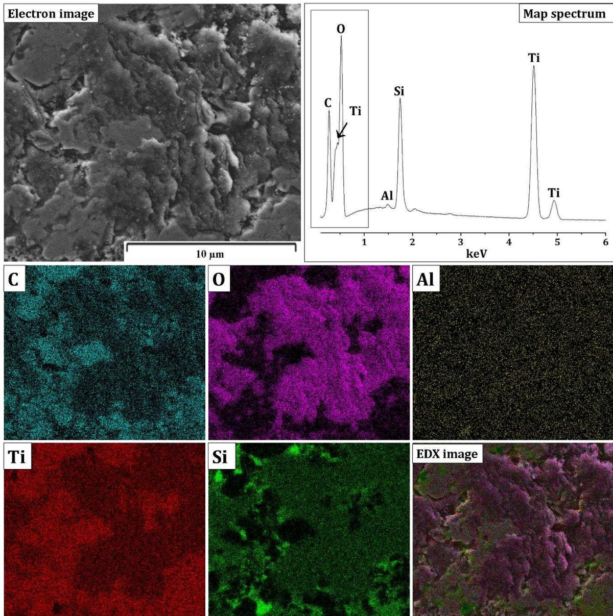
**Fig. 8.** EDX elemental distribution map and spectrum inside the wear track of Maxthal 312-TiC/Al<sub>2</sub>O<sub>3</sub> worn section from wear condition 100 rpm / 60 min.
