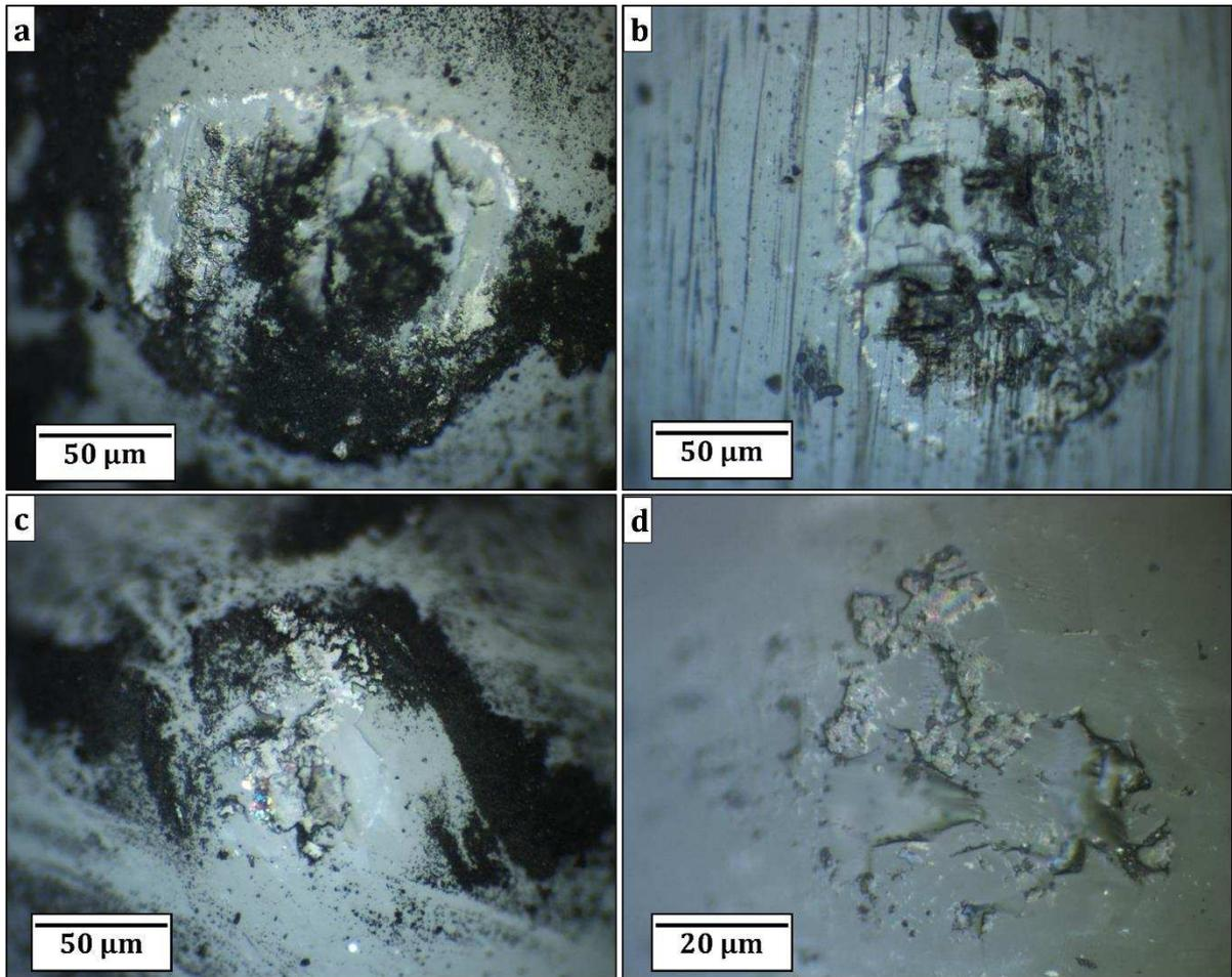
**Fig. 12.** Optical images of the  $\text{Al}_2\text{O}_3$  ball surface after unlubricated sliding against the Maxthal 312 disc ((a) before cleaning and (b) after cleaning) and Maxthal 312-TiC disc ((c) before cleaning and (d) after cleaning) discs for the contact condition 100 rpm for 60 min.
