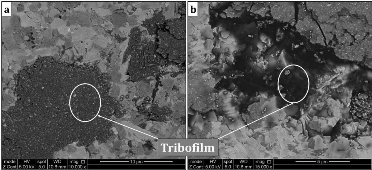
**Fig. 13b.** SEM micrographs of the pre-transition phase of the Maxthal 312-TiC/Al<sub>2</sub>O<sub>3</sub> sliding surface.
