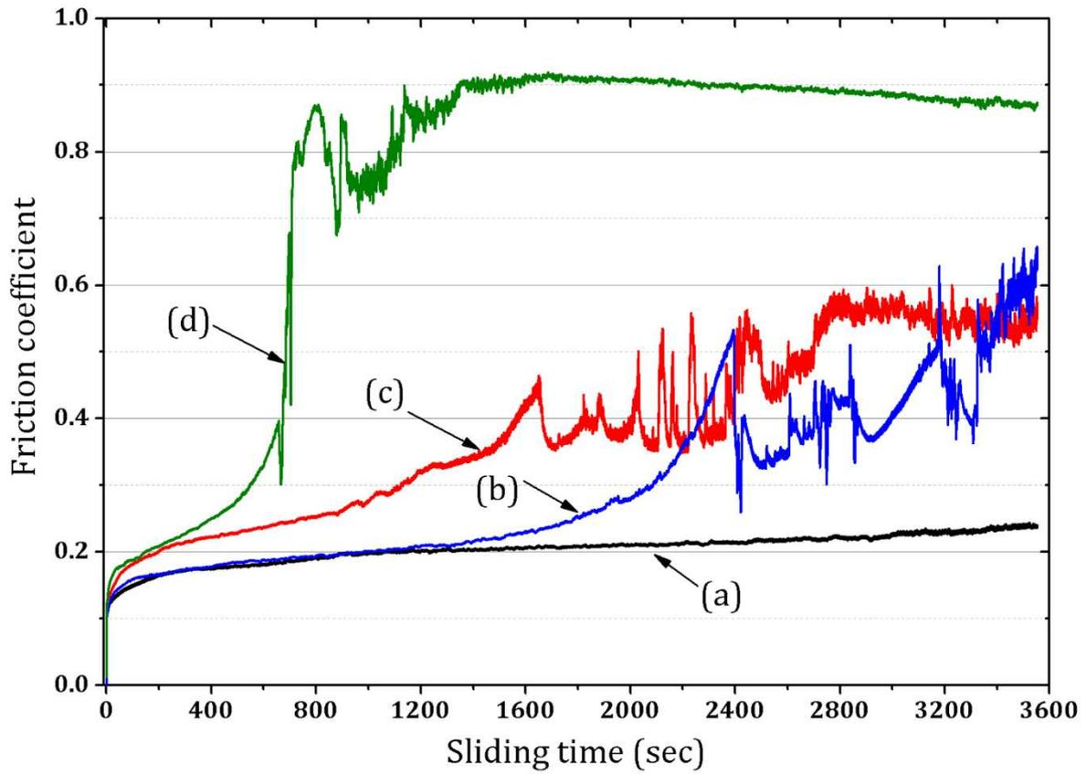
**Fig. 5.** The evolution of friction coefficients of the bulk samples upon sliding against  $\text{Al}_2\text{O}_3$  ceramic using a constant normal load of 0.5 N: (a) Maxthal 312-TiC (50 rpm / 60 min), (b) Maxthal 312 (50 rpm / 60 min), (c) Maxthal 312-TiC (100 rpm / 60 min), and (d) Maxthal 312 (100 rpm / 60 min).
