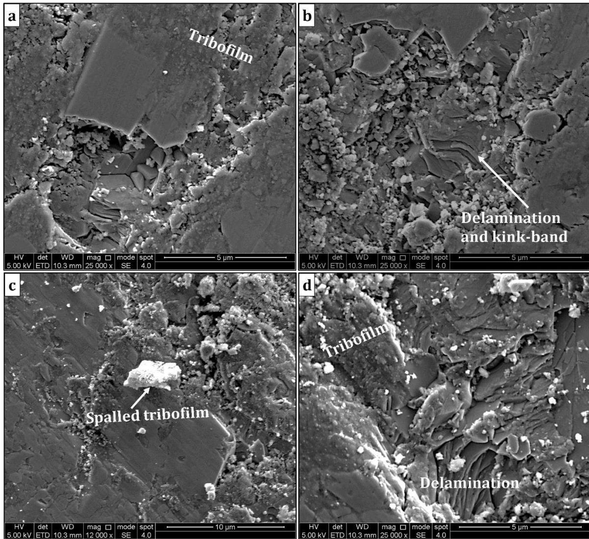
**Fig. 14.** SEM micrographs of the sliding surface of Maxthal 312/Al<sub>2</sub>O<sub>3</sub> for the contact condition 50 rpm for 60 min (a-b), and 100 rpm for 60 min (c-d). Note: white bits are spalled tribofilms.
