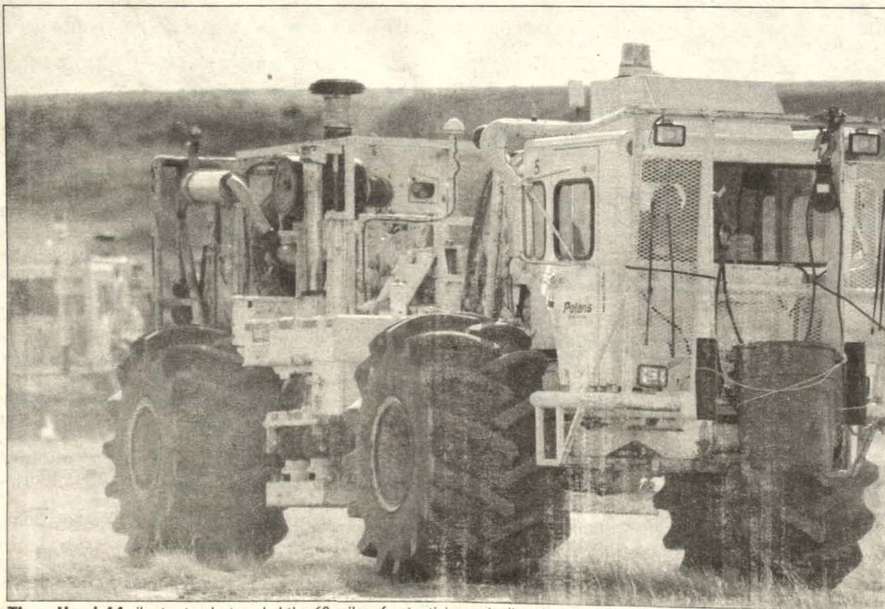
These Hemi-44 vibrator trucks traveled the 60 miles of potential gas pipeline sites, stopping every 50 feet to lower a tabletop-sized vibrator and send shockwaves into the ground.
