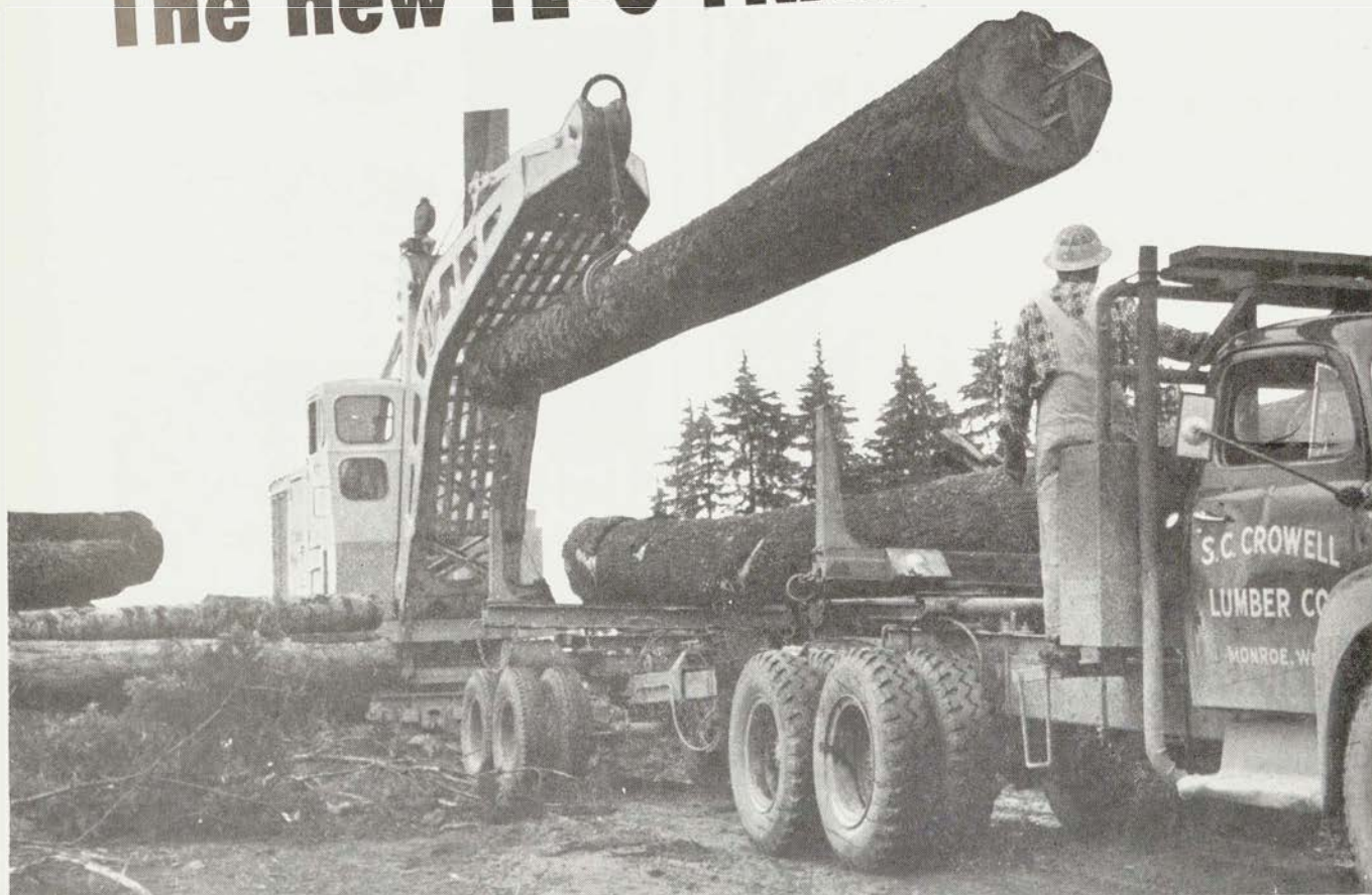
One of the first of the new TL-6 Washington Trakloaders loads medium sized logs for S. C. Crowell near Sultan, Washington.
