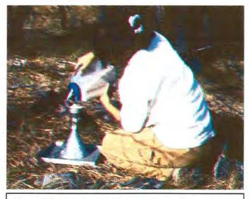
Figure 3.5. Pouring sand into sand cone apparatus.
