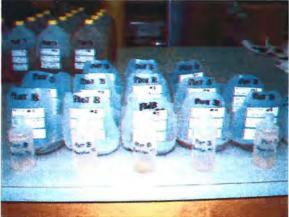
Figure 3.22b. Front view of cut milk jugs and suspended sediment sub-samples.
