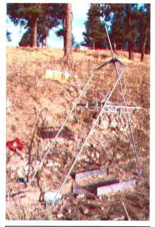
Figure 3.10. Simulator setup with materials: simulator, metal tripod, water source, battery, metal panels collection jug.
