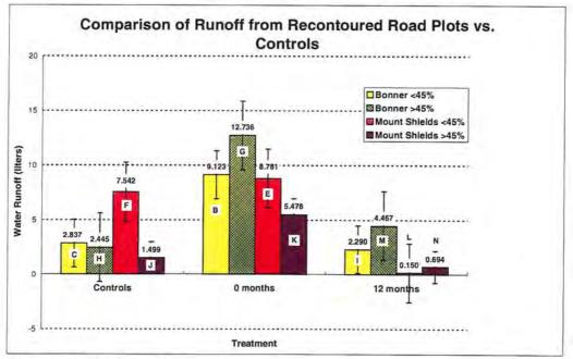
Figure 4.13. Water runoff comparison on recontoured road plots vs. controls
