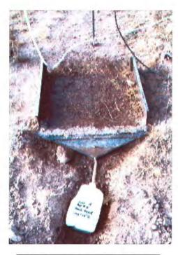
A triangular piece of metal was used for the fourth side of the square plot. The triangular piece had tubing attached to its bottom point where the runoff was to escape. The long edge of the triangular piece closed off the square box. The long side was sealed with bentonite (Figure 3.11) where the metal edge was driven into the ground. The other two sides of the triangle had raised edges, which prevented the runoff from flowing off
