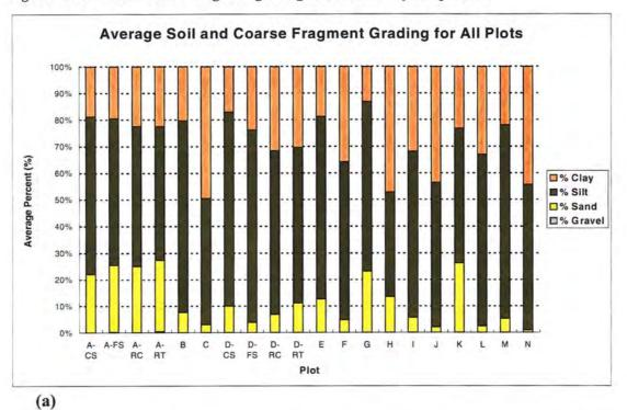
Figures 4.15. Soil and coarse fragment grading and silt and clay comparisons
