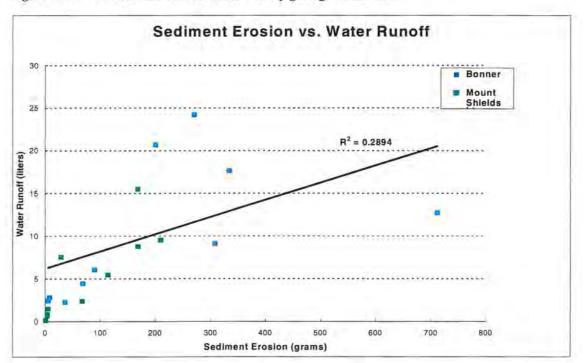
Figure 4.11. Sediment and runoff correlation by geologic formation
