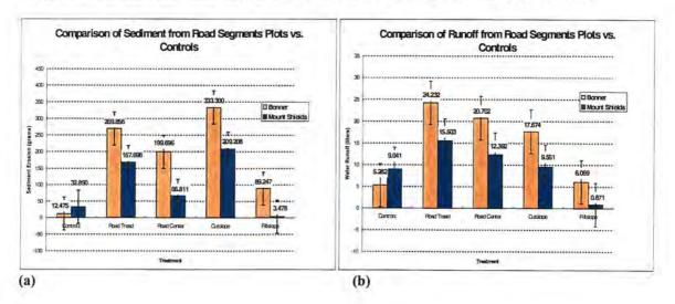
Figure 4.14. Erosion and runoff comparison of road segments (Standard error bars shown)
