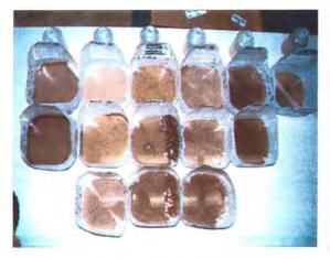
Figure 3.22a. Top view of cut milk jugs containing sediment erosion only (without runoff).
