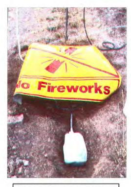
Figure 3.15. Sign used to cover plot until constant rain was established. collected from the 25 water usage tests was 27.78 liters with a standard deviation of 0.36. Under these established specifications, approximately 2.84 (1.12 inches) of water "rained" on each plot in the field.
