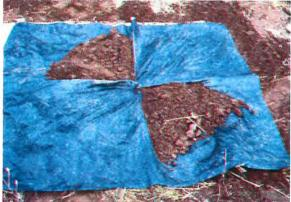
(d). Opposite sides were removed, using a paint brush to remove any fines.
