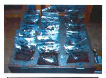
Figure 3.16. In-place (bulk) density samples.
