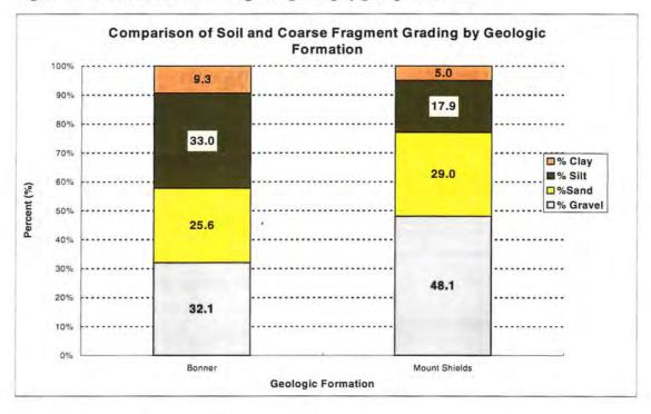
Figure 4.7. Textured and coarse fragment grading by geologic formation
