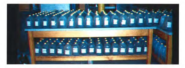
Figure 3.20. All sediment and runoff samples collected. The number of jugs per site was dependent upon the treatment conducted on the site.
