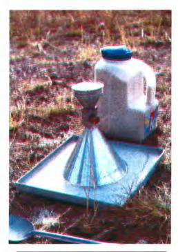
Figure 3.3. Sand-cone apparatus.
