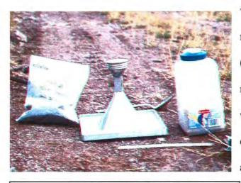
was removed from the hole using a metal spoon and placed in a plastic bag (see Figure 3.4 left). The material removed from the test hole was weighed in the field, as was the sand container and sand. The sand-cone apparatus was then placed on the metal plate, with the valve securely closed.
