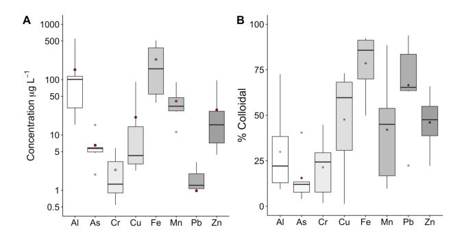
Figure 2. Boxplot represent the first quartile, median, and third quartile, red dot represents the mean, whiskers represent minimum and maximum values. A) Comparison of metal(loid) concentration across all terminal lagoons. B) Comparison of percent colloidal of all elements in the terminal lagoons of all field sites. N=6 for all elements except n=5 for Cr and n=4 for As.
