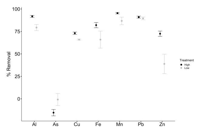
Figure 11. Percent metal(loid) mass removal. Black points represent high treatment and grey points represent low treatment. Error bars represent the standard error.
