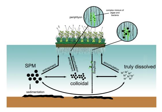
Figure 12. Conceptual model displaying the observed pathways of metals in this FTW mesocosm experiment.
