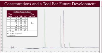
(Above) A HPLC method developed to determine concentration of the compounds used in this study. Results showed 100% recovery with most compounds, the lowest observed value being 87%. The above method worked universally for the studied compounds and allows for determination of LogP for future studies. Determination of LogP allows for greater accuracy in determining the best solvent to use for a formulation.
