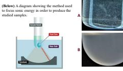
(Above, Right: A, B) An example of the dispersions prepared via traditional bath sonication shows settling and aggregation of particles, while (Above, Right: B) the same dispersion prepared via focused ultra-sonication resulted in a uniform suspension.
