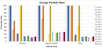
(Above) Average particle sizes for suspensions of the studied compounds in a variety of solvents. Samples were tested at day 0 and day 14 or 21 after being kept between 2°C-8°C to determine changes in particle size over time. Sizes under 200 nm are desirable as this allows for sterile filtration; the majority of compounds resulted in a formulation with initial particle sizes below 200 nm.
