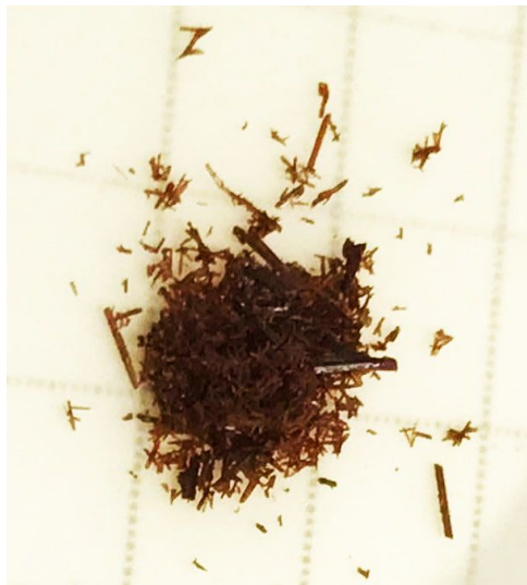
Figure 3. Cr(III)-Salen crystals, synthesized as described by Sugden et al. (2001).
