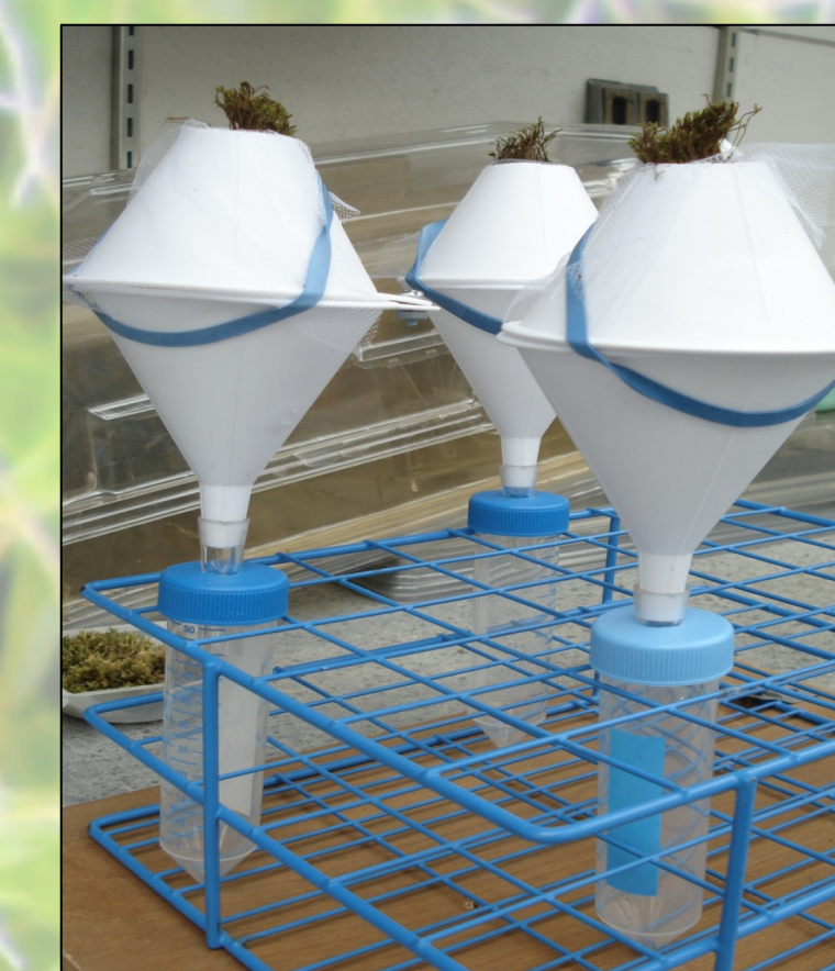
Leachate Collection Units: Dehydrated moss is placed on top and watered. Leachate throughfall is collected below.
