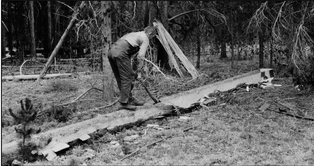
Figure 4. A Tie Hack Cutting the Face of a Railroad Tie (USDA Forest Service, 2018). This photo is credited to Kenneth D. Swan. The date for this photo is August 12, 1924. In addition to the broad axe in use by the worker, one can see his hand saw and a bark scraper on the ground at the right edge of the photo.
