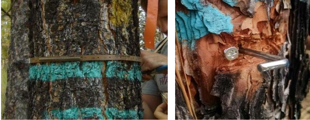
Figure 2.1 (Left) UMS Dendrometer D1 Vernier band dendrometer (Right) Reineke hook-and-screw point dendrometer
