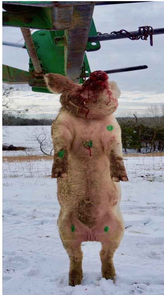
Figure 3: Pig A hanging upright from tractor and hayfork with green livestock marker on areas selected for impact with AR-15
