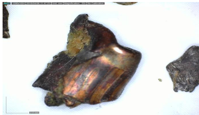
Figure 29: One of the largest bullet fragments recovered from Fig A, which has been magnified using the Dino-Lite to show the outer copper coating and rifling (image from Dino-Lite)
