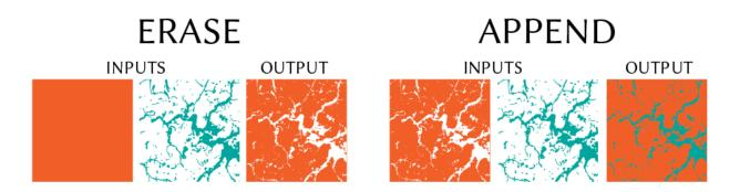
*Figure 11.* A graphic representation of the process for erasing and appending multiple land cover class feature classes.
