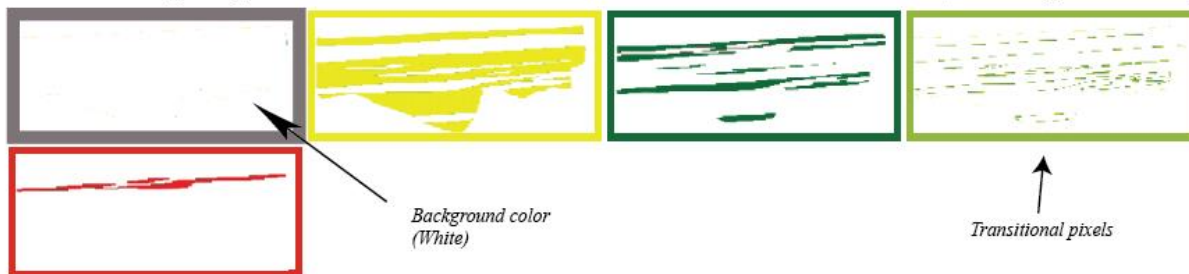
Figure 7: Facies quantification process. Top left: Measured sections and high-resolution photos constrained facies maps at all outcrops. Maps were imported into the image analysis software, which calculated image statistics, including color proportions. Facies proportions were normalized for the three primary map facies and their respective colors. Background colors such as white (39.94% in this example) were disregarded, and percentage values of transitional pixel clusters (i.e. “avocado”) were split between the two primary colors (yellow and green). This process was repeated for each zone of the geomodel at all outcrops, and provided the primary statistical input for facies proportions and spatial trends
