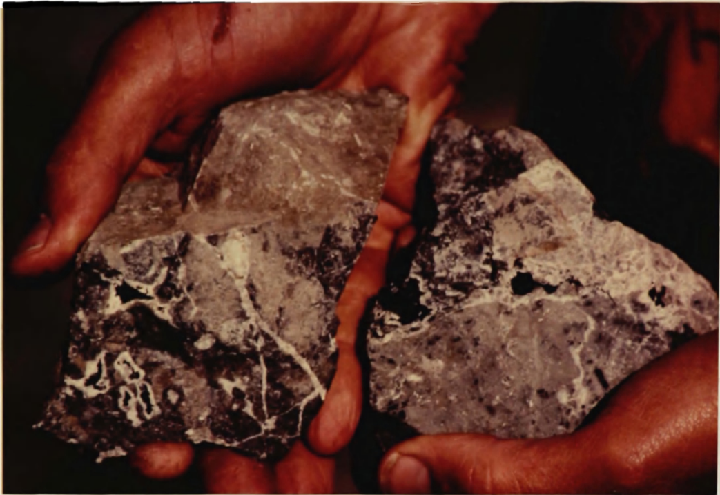
Fig. 25a. Black pyrobitumen enclosed within white dolomite and calcite veinlets crosscutting Devonian dolostone at Copper Hill.
