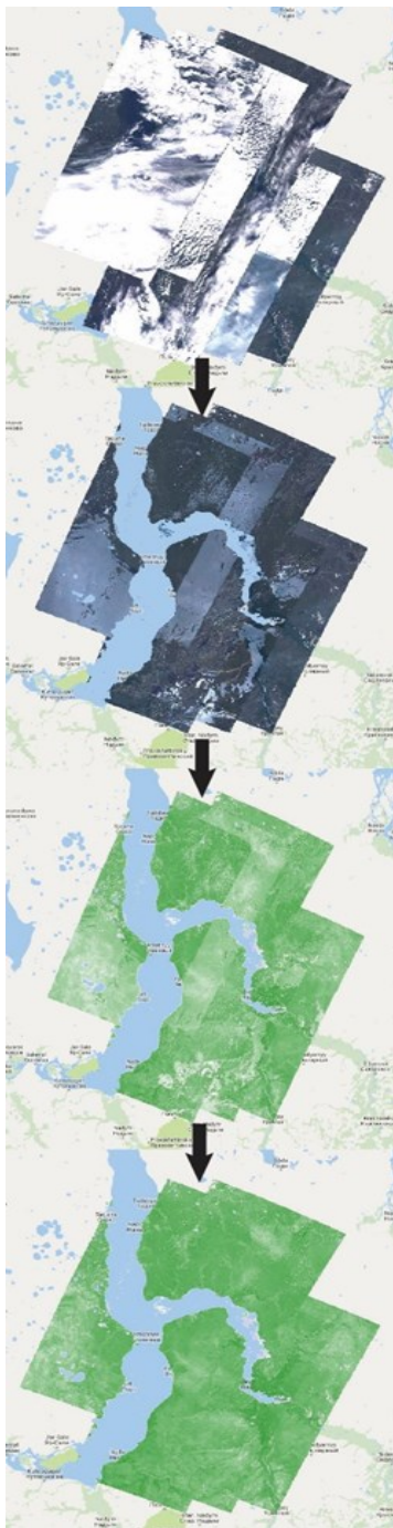
Figure 5. Illustration of mosaicking the imagery together based upon the maximum seasonal NDVI value. First all imagery within the growing season are selected. Clouds and water pixels are then masked out (second tile). NDVI was then computed for all images (third tile). Finally, a mosaic is created by selecting the maximum NDVI value per pixel from the stack of images.
