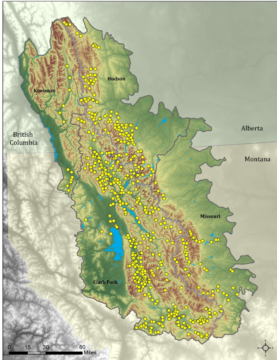
Fig. 1 Stream temperature monitoring sites ( N = 743 sites) in the Crown of the Continent Ecosystem, USA and Canada. Temperature was measured using digital thermographs (Hobo and Tidbit models; Onset Computer Corporation, Pocasset, Massachusetts, USA; accuracy \pm 0.2^{\circ}\text{C} ) that recorded temperatures at bi-hourly or hourly intervals
