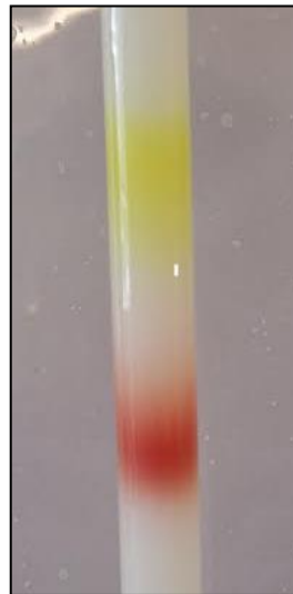
Figure 2.2 G-25 size exclusion chromatography of Hu Cyt c . Yellow band is ferricyanide. Red band is cytochrome c .
