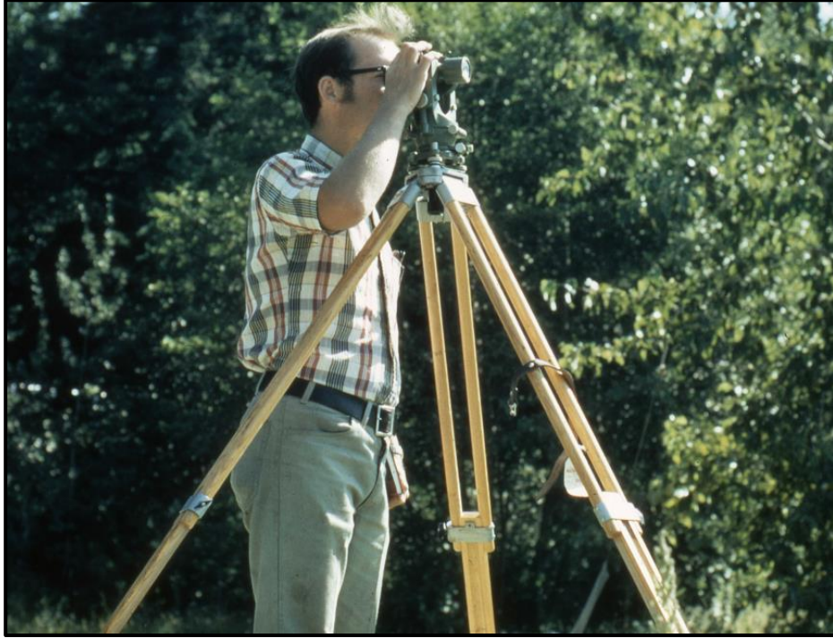
Figure 5. Shore-based theodolite station mentioned by Wold (1982). A notebook can be seen in the surveyor's left hand. The notes from any theodolite readings from shore or sextant readings from the survey boat are lost. (Image scanned from a slide provided by Richard Wold.)
