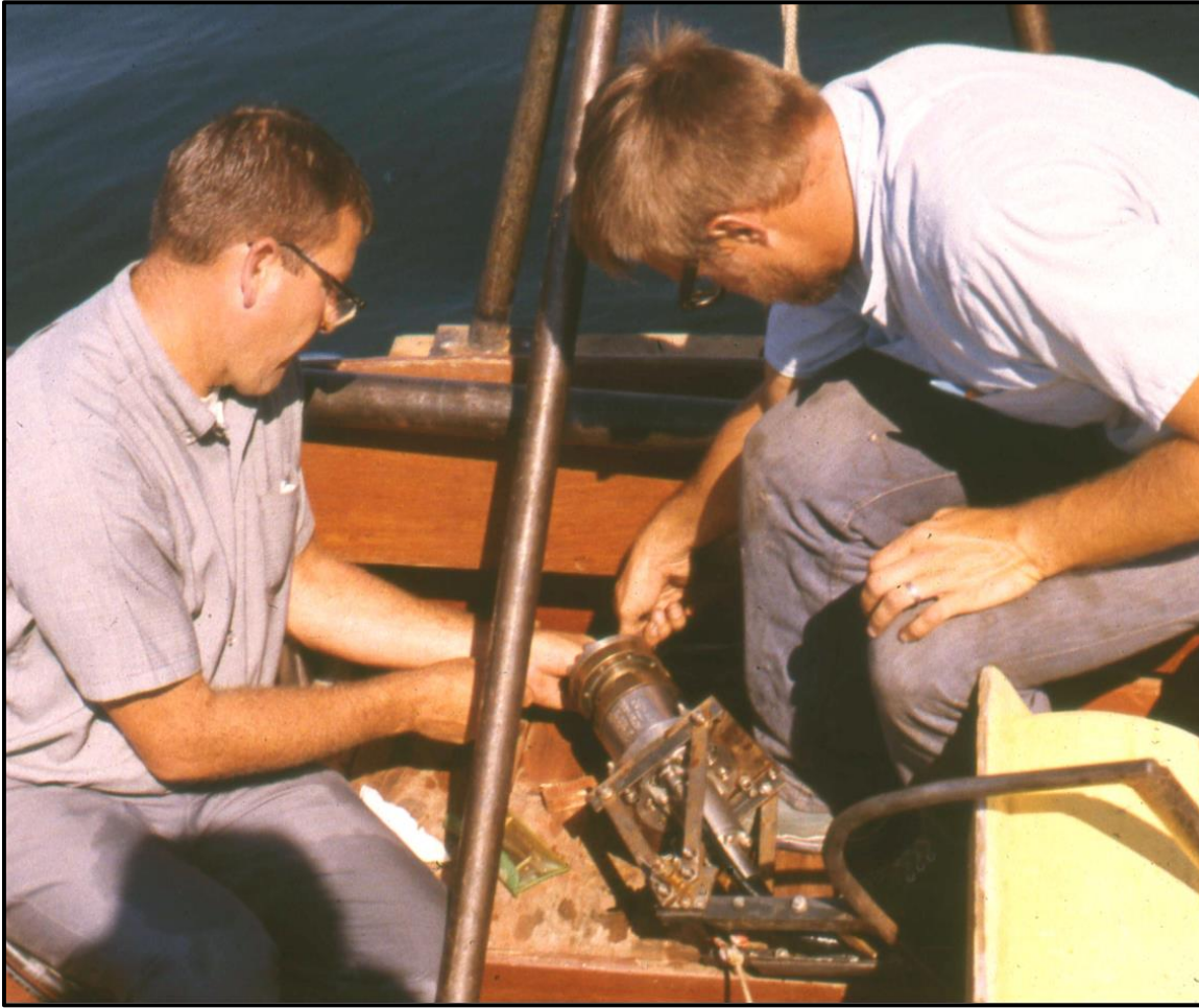
Figure 2. Performing maintenance on the air gun. The air gun is the metal device on the deck in the lower, center of the image. (Image scanned from a slide provided by Richard Wold.)
