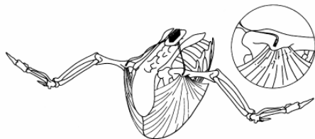
FIG. 2. Attachment site of the strain gauges on the delto-pectoral crests, and back-plug position (inset).
