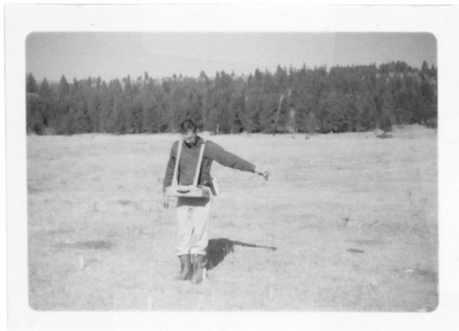
Figure 8. This shows the sampling procedure which was employed throughout the study. The radiometer was carried in the canvas case with shoulder straps. Much of the time a tape recorder was used for recording the data.
