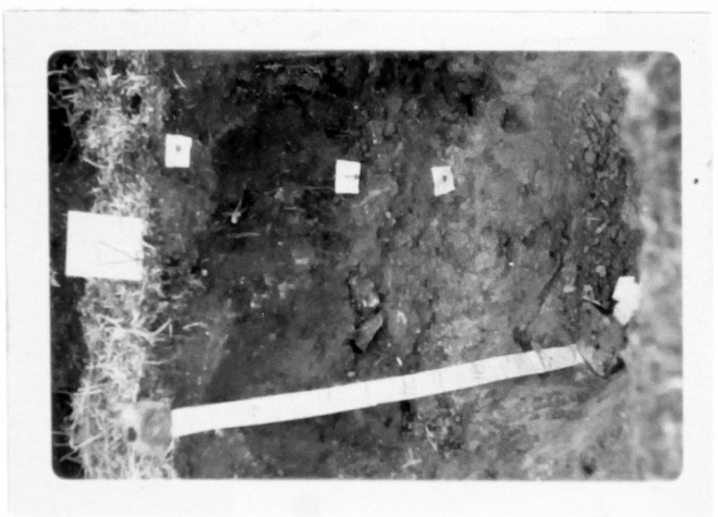
Figure 6. Soil profile photograph for site V. See Table 4 for description of horizons. This is a humic gley soil profile.
