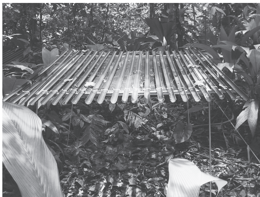
PLATE 1. An example of the enclosures constructed to manipulate throughfall and to impose the experimental drought. Photo credit: W. R. Wieder
