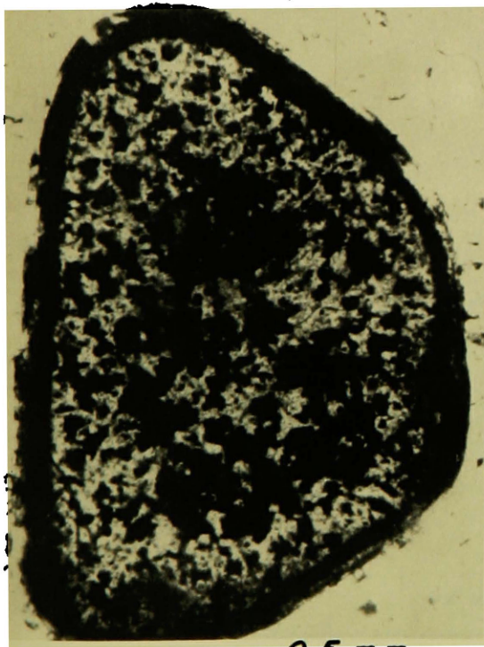
Figure 3. Phosphorite grains in thin section, illustrating varied distribution of inclusions within individual grains
