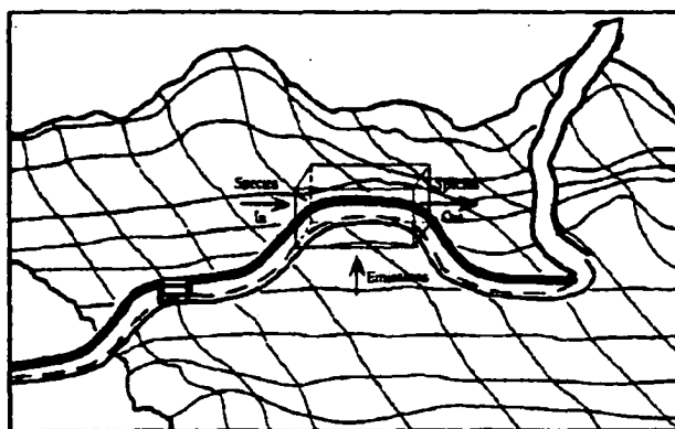
Figure 8.8 Schematic of the basic scenario for modeling the influence of the city on the smoke plume. Illustration shows simulation starting with the packet, initially containing biomass combustion emissions, being advected into an urban airshed and remaining for some period of time before being advected out. Notice that the moving packet only covers a portion of the fixed urban box model at any given point in time. [Adapted from Seinfeld and Pandis, 1998].
