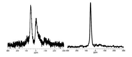
Figure 1. (left). <sup>27</sup>Al MAS-NMR spectra for siliceous sinter from TG, Geyser Valley, Kamchatka. (right). <sup>27</sup>Al MAS-NMR spectra for siliceous sinter from an YSS, Shoshone Geyser Basin, Yellowstone National Park,
