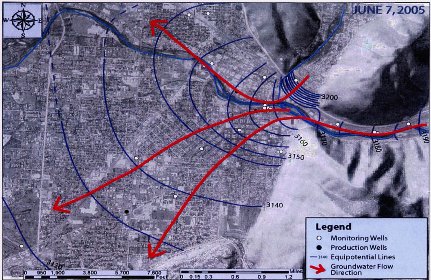
Figure 6. Groundwater flow for the Missoula Valley. Flow is to the southwest on the southern side of the Clark Fork River, and to the northwest on the northern side of the river. Note the steep gradient in the mouth of the Rattlesnake drainage.
