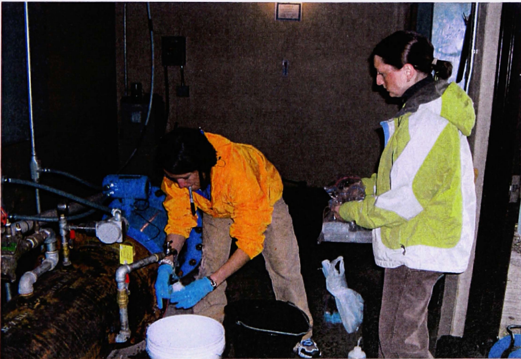
A4. Ultra clean sampling of one of Mountain Water Co.'s production wells. Robyn (left) is "clean hands" and Amelia (right) is "dirty hands."
