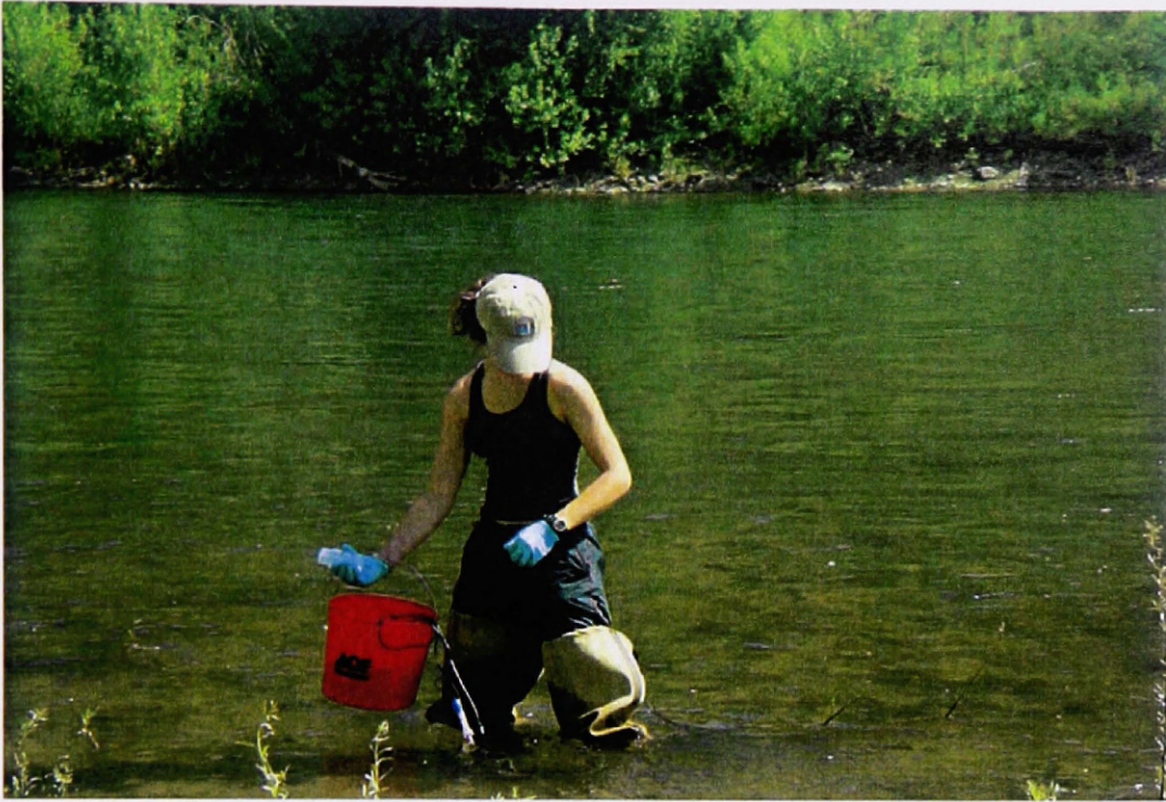
A3. Measuring pH, temperature and conductivity in the Clark Fork River.
