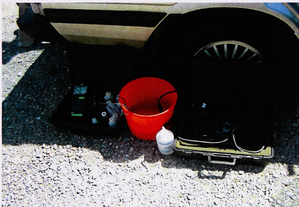
A2. Measuring pH, temperature and conductivity at a well site. The red bucket was filled from water in the pump rather than from a bailer.
