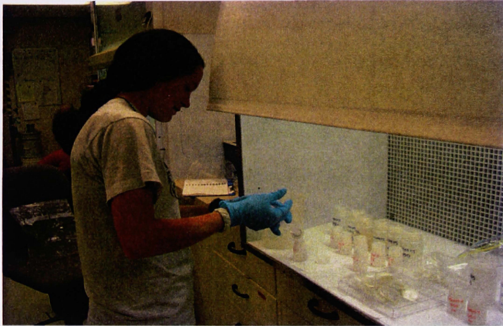
Figure 8. Ultra-clean filtering in the hood. Filtering with <0.45\mu\text{g} filters and acid washed syringes.
