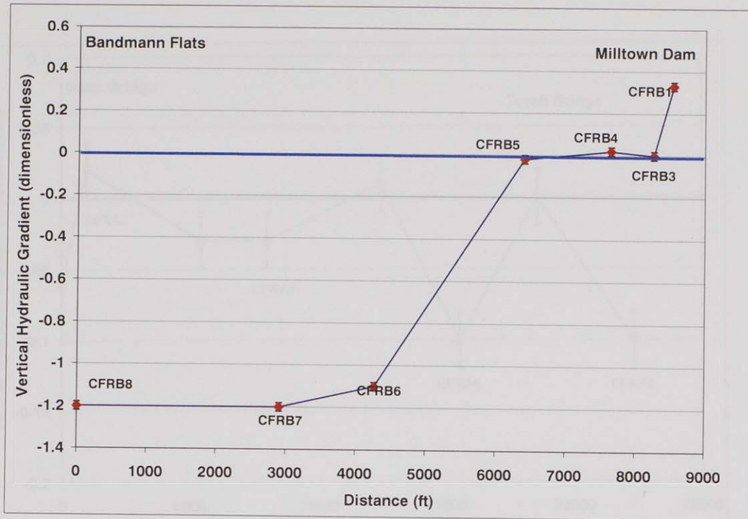
Figure 46 The distribution of vertical hydraulic gradients below Milltown Dam. Negative gradients indicate zones of river water seepage to the underlying groundwater systems. Positive gradients are present when groundwater is discharging to the river bed. Areas with no measurable upward or downward gradients suggest no measurable exchange of water between systems is occurring. The gradients were collected between August and October 2006. The error bars show the measurement error.
