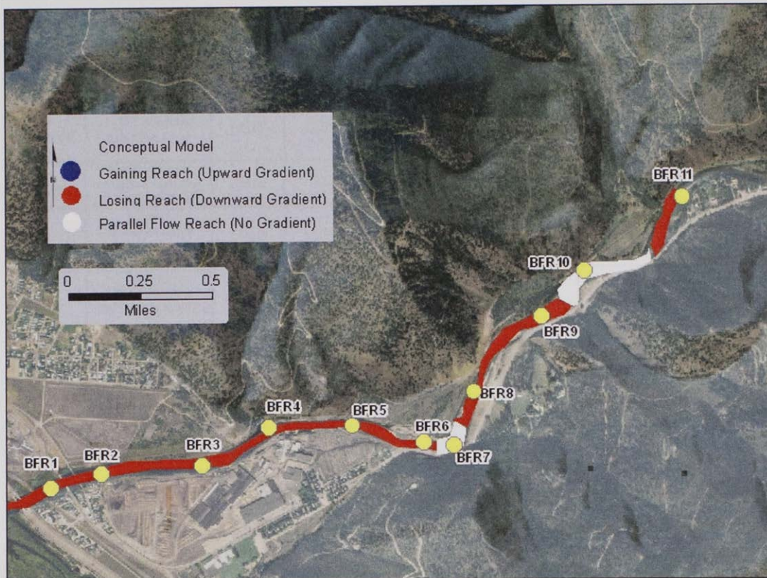
Figure 55 Conceptual distribution of vertical hydraulic gradients on the Blackfoot River above Milltown Dam. Negative gradients indicate zones of river water seepage to the underlying groundwater systems. Positive gradients are present when groundwater is discharging to the river bed. Areas with no measurable upward or downward gradients suggest no measurable exchange of water between systems is occurring. These are considered areas of parallel flow. The conceptual model was determined for low water conditions.
