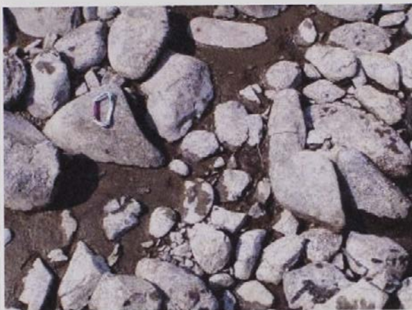
Figure 52 A picture of the riverbed sediments below Milltown dam. The photo shows the coarse river bed armored with fine grained reservoir sediments.
