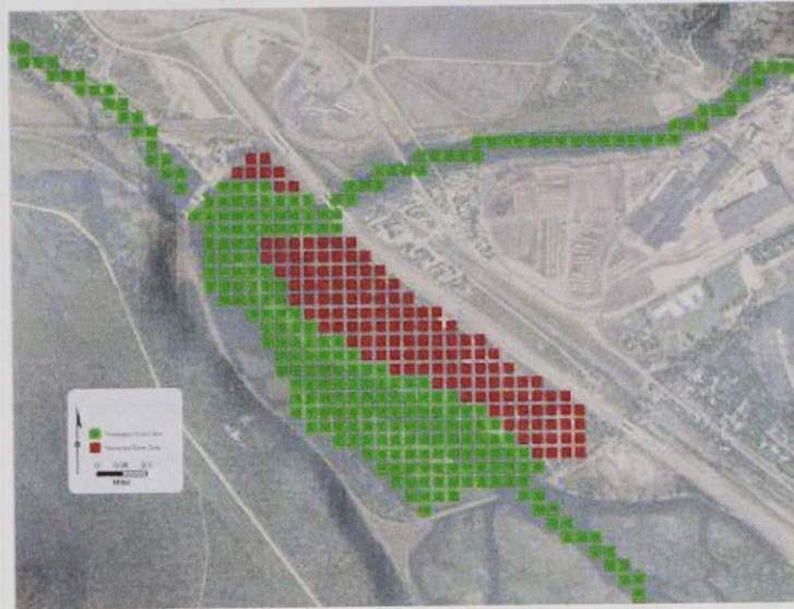
Figure 61 Map of the river cells removed from the reservoir to simulate lower leakage from construction sediment dewatering and sediment removal.
