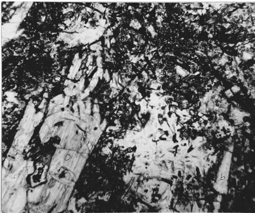
Figure 2: Type V rock; shows serpentine pseudomorph after olivine (o), magnetite & ilmenite (opaque), apatite needles (clear), and both light and dark glassy groundmass. Plain light, x 50.
