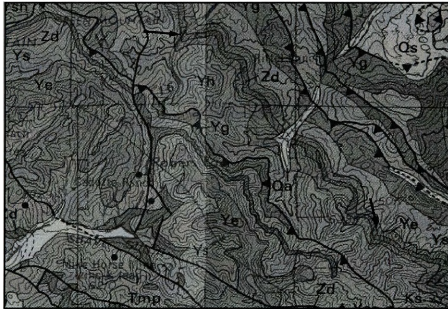
Figure 17. The trace of a sill "Zd" from sample site RPE (north arrow) to the Wolf Creek site (south arrow). (Map by Mudge et al., 1982).
