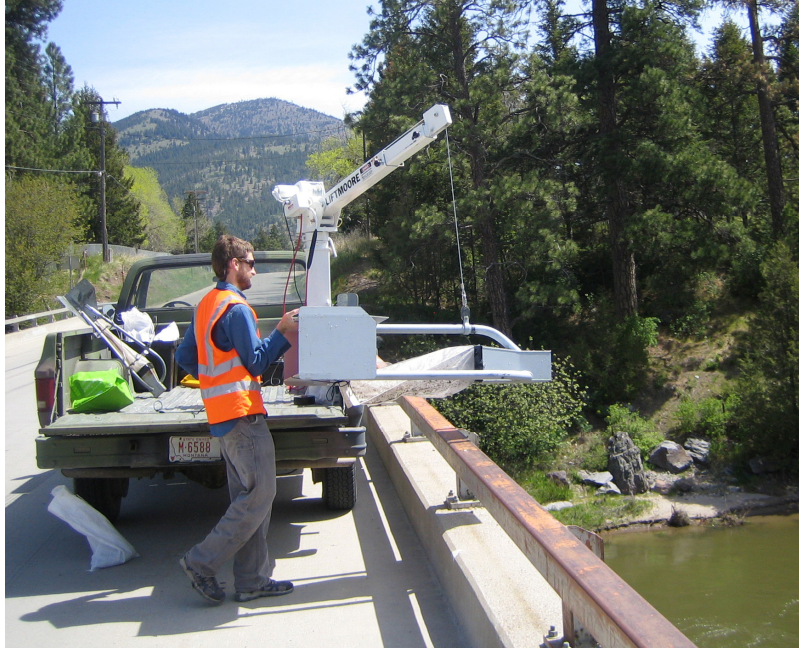
Figure 2.3 Sampling in 2009 with the Toutle sampler from Deer Creek Bridge.
