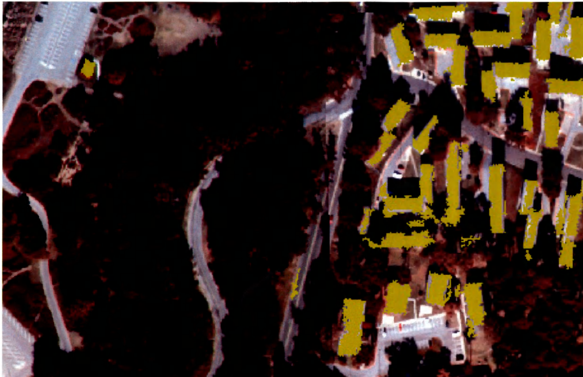
Figure 24: Final training image building detection classification. every building is identified
