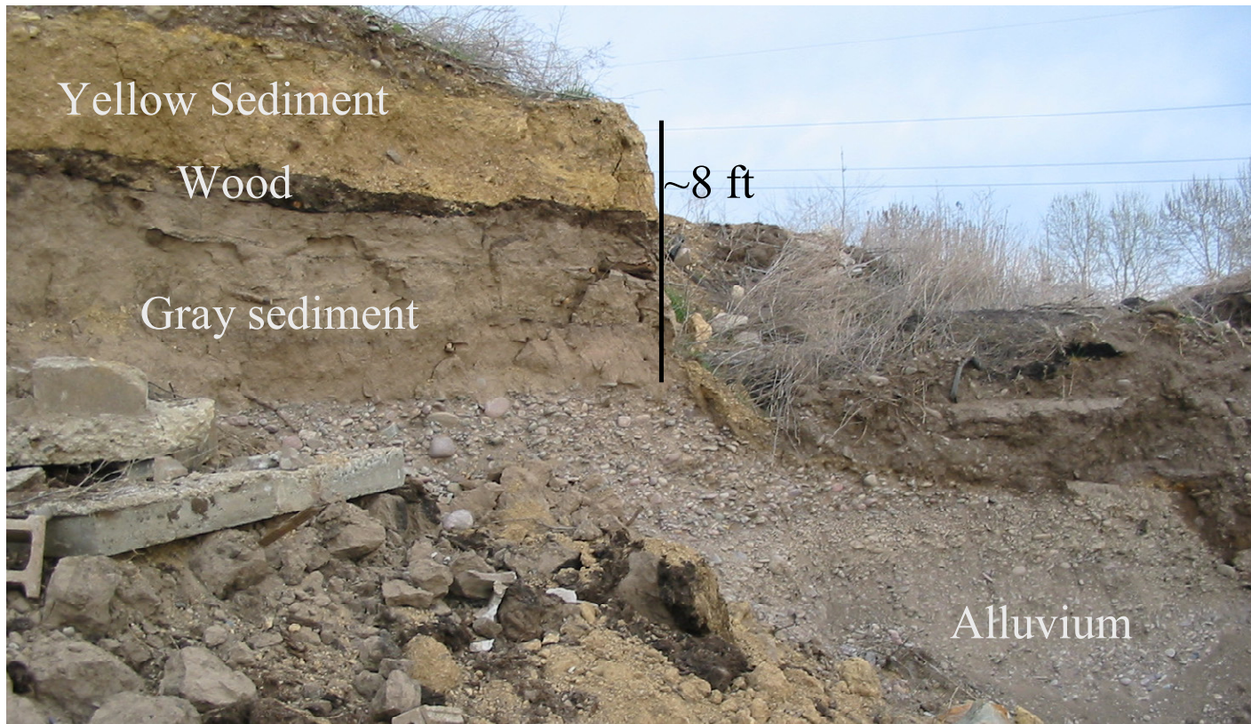
Figure 6 Subsurface layering at Eko Compost.
