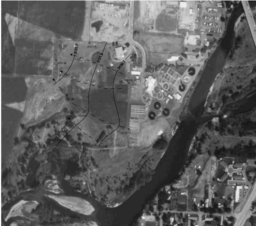
Figure 13 January 11, 2006 Potentiometric map of the water table surface at Eko Compost. .
