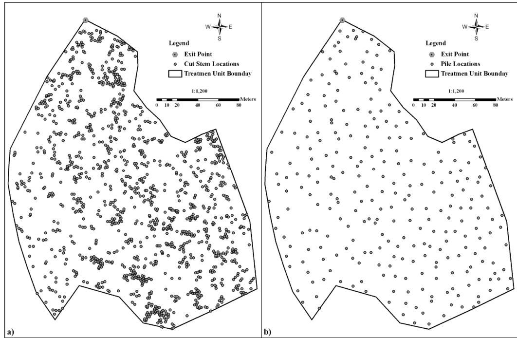
Figure 2.12. Cut-tree locations under thinning scenario II (a), and the corresponding log-pile locations identified by the log bunching algorithm (b).
