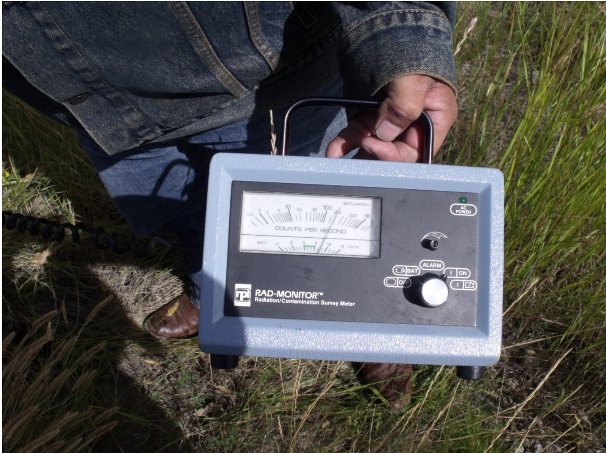
Figure 5.2. A reading of 200 cps at the protruding concrete slab of the “old dozed site”.
