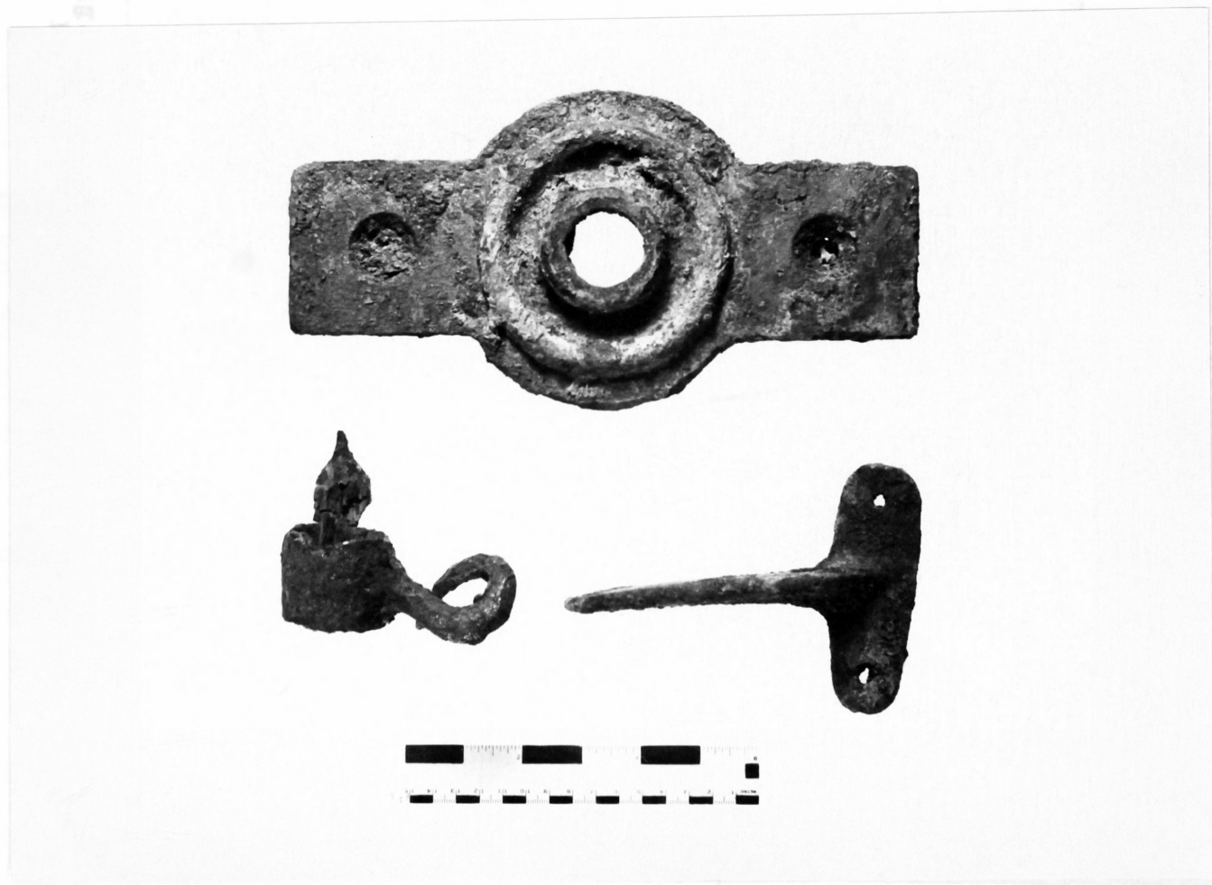
Fig. 14.--Wagon and Buggy Parts. Top, Bolster Iron; Bottom Left, Single Tree Iron; Bottom Right, Buggy Step and Foot Rest
