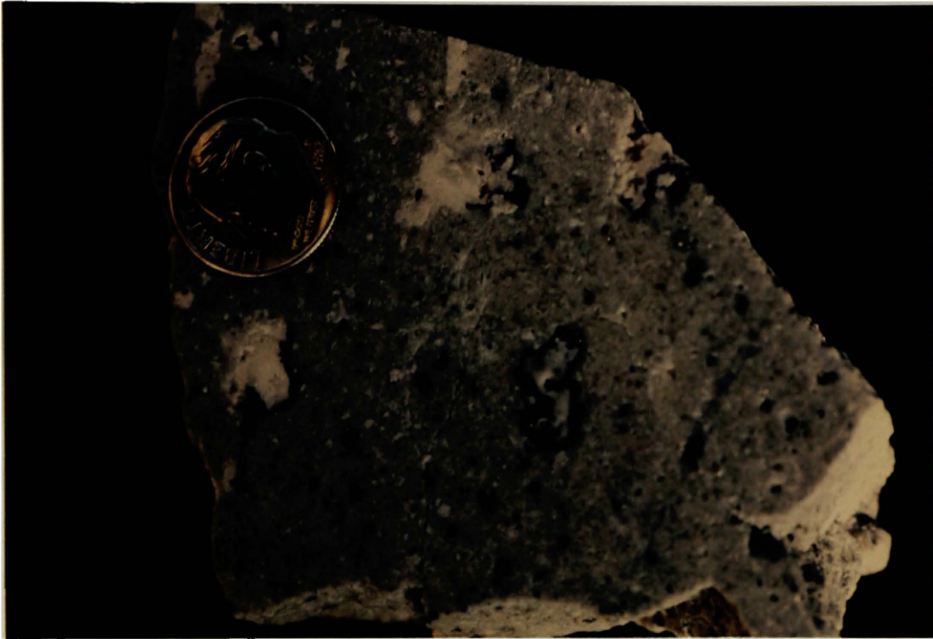
Figure 22: Photograph of disseminated sphalerite (brown) and finer-grained pyrite (brassy) in quartz-sericite altered andesite.
