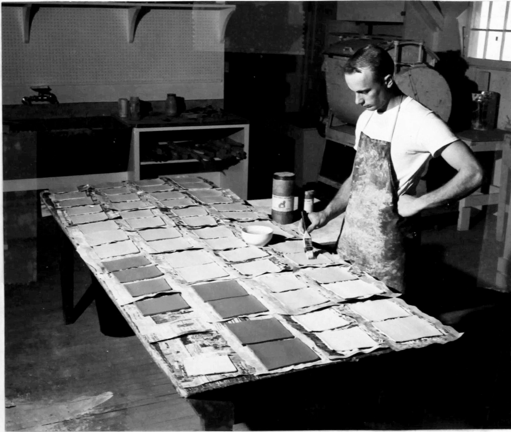
The second coat of glaze was applied after the first coat dried, usually in fifteen minutes. If engobe colorants were used, they were allowed to dry, and then the glaze applied.
