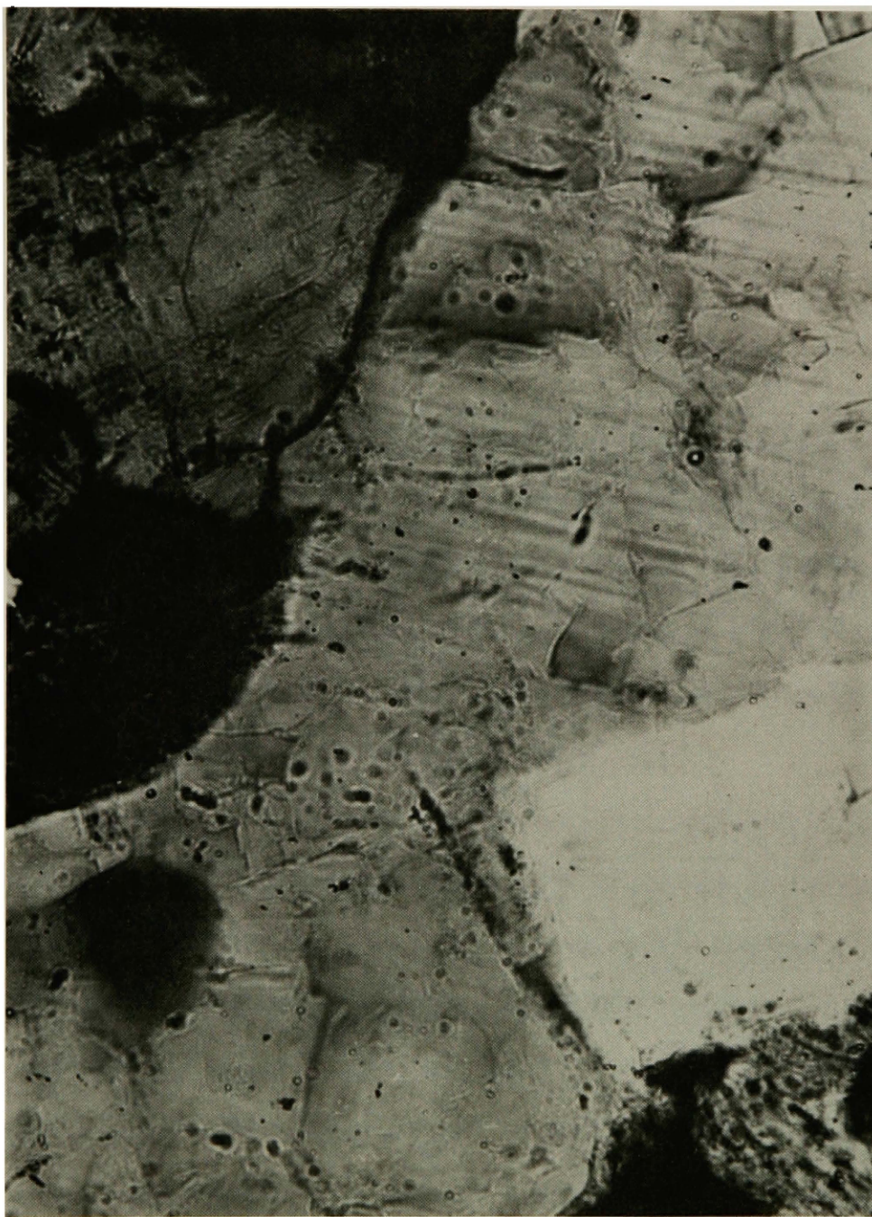
Plate 15. Photomicrograph of deformation lamellae in quartz, sample RL-19. Field of view (long dimension) is 0.9 mm.
