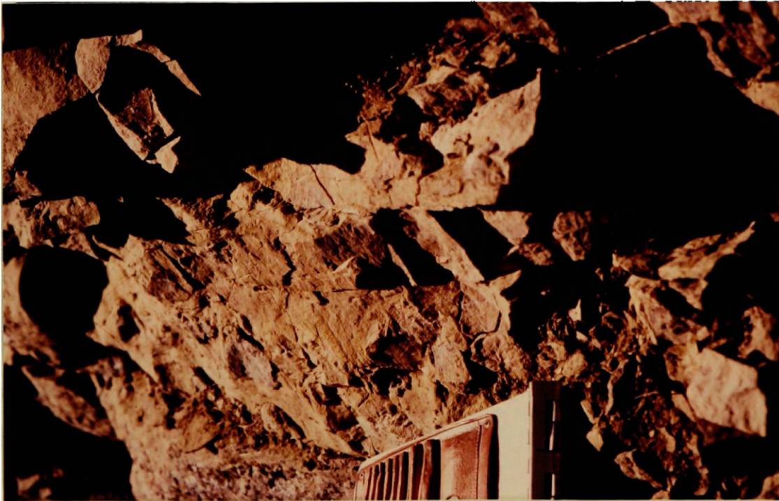
Figure 22.--Limestone breccia, lower Upper Limestone, Hogback Mountain. Limestone patches less than 3 in. in diameter. Notebook for scale. Up to upper right of photo.
