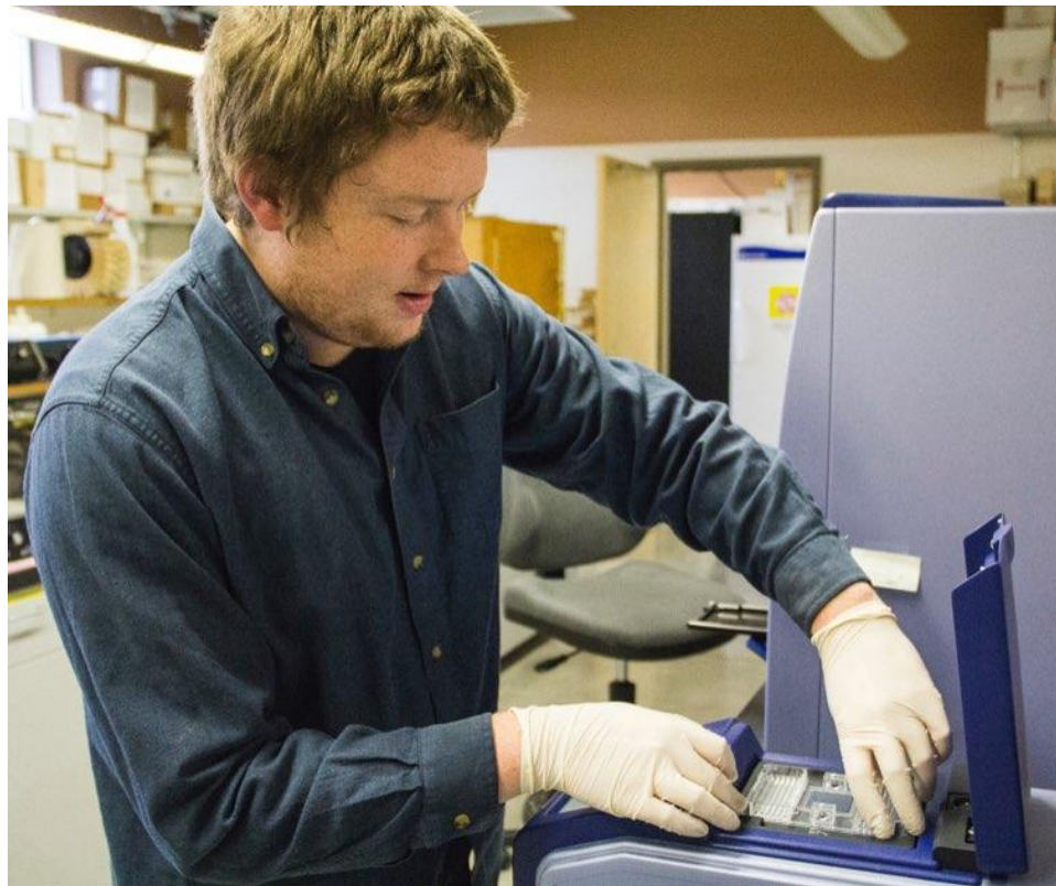
Seth Smith inserts the chip into the PCR machine. After several hours the data appears on the screen.
