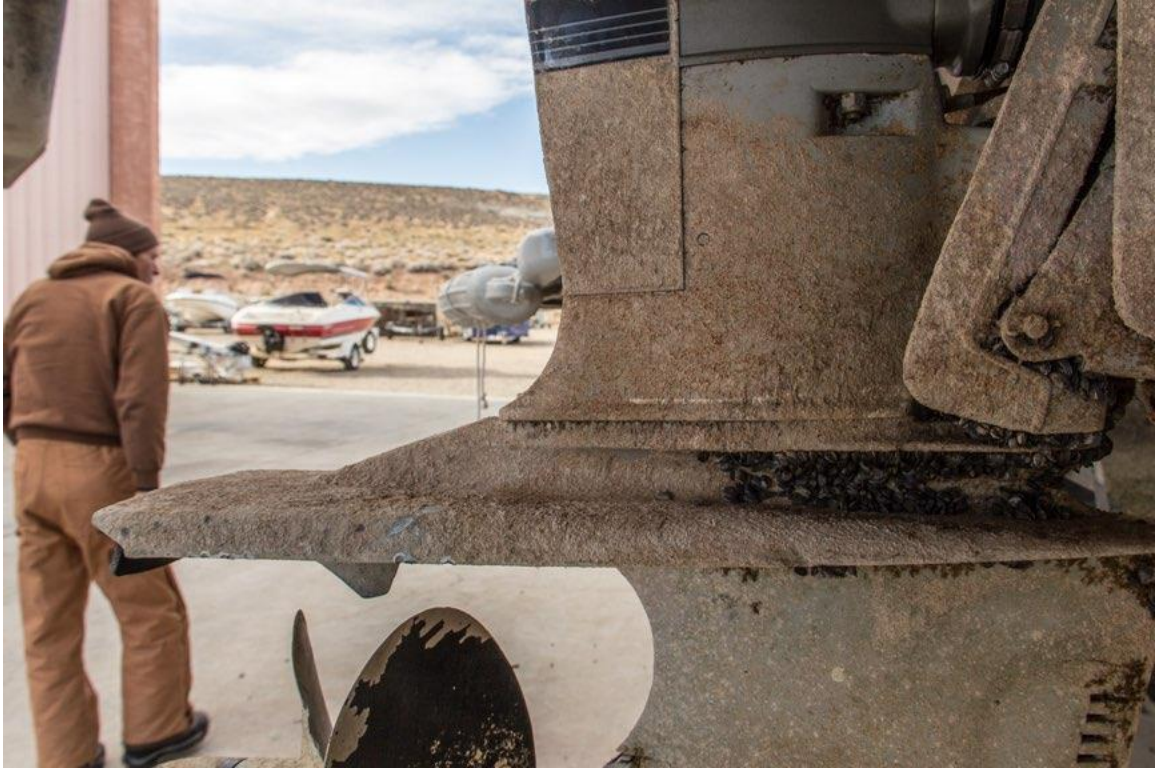
Wayne Gustaveson looks at rental boats near Wahweap Marina for signs of mussels. Lake Powell has an incredible number of boats. Many of the large houseboats that stay in the water or in storage for the winter must be cleaned once or twice a year to reduce buildup of mussel colonies.
