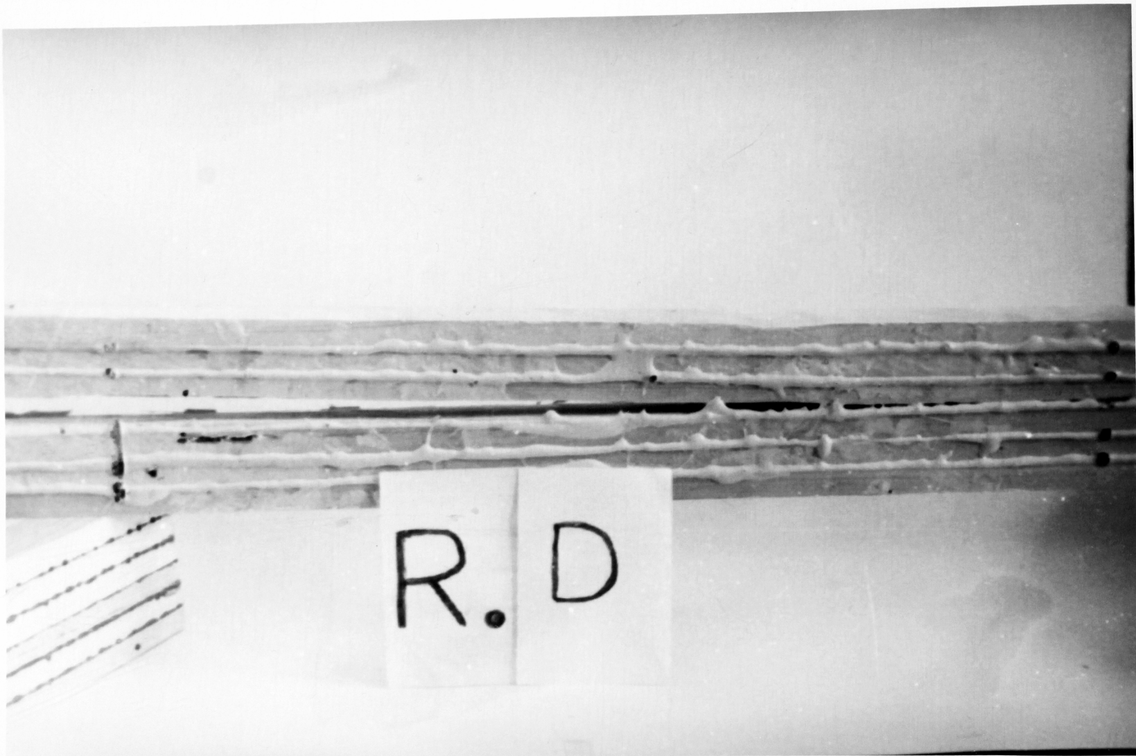
FIGURE VI TYPICAL FAILURE OF THE REINFORCED BEAMS, TYPE D
