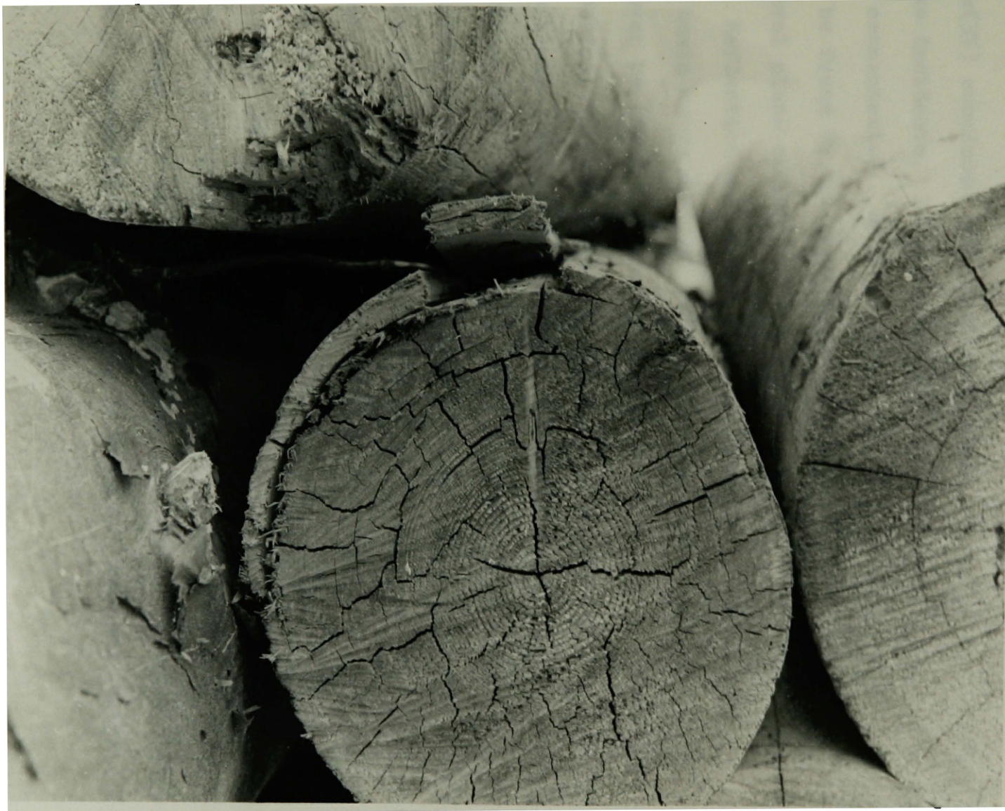
FIGURE 24. RING SHAKE AT THE SAPWOOD-HEARTWOOD JUNCTION OF A DOUGLAS-FIR SAWLOG.
