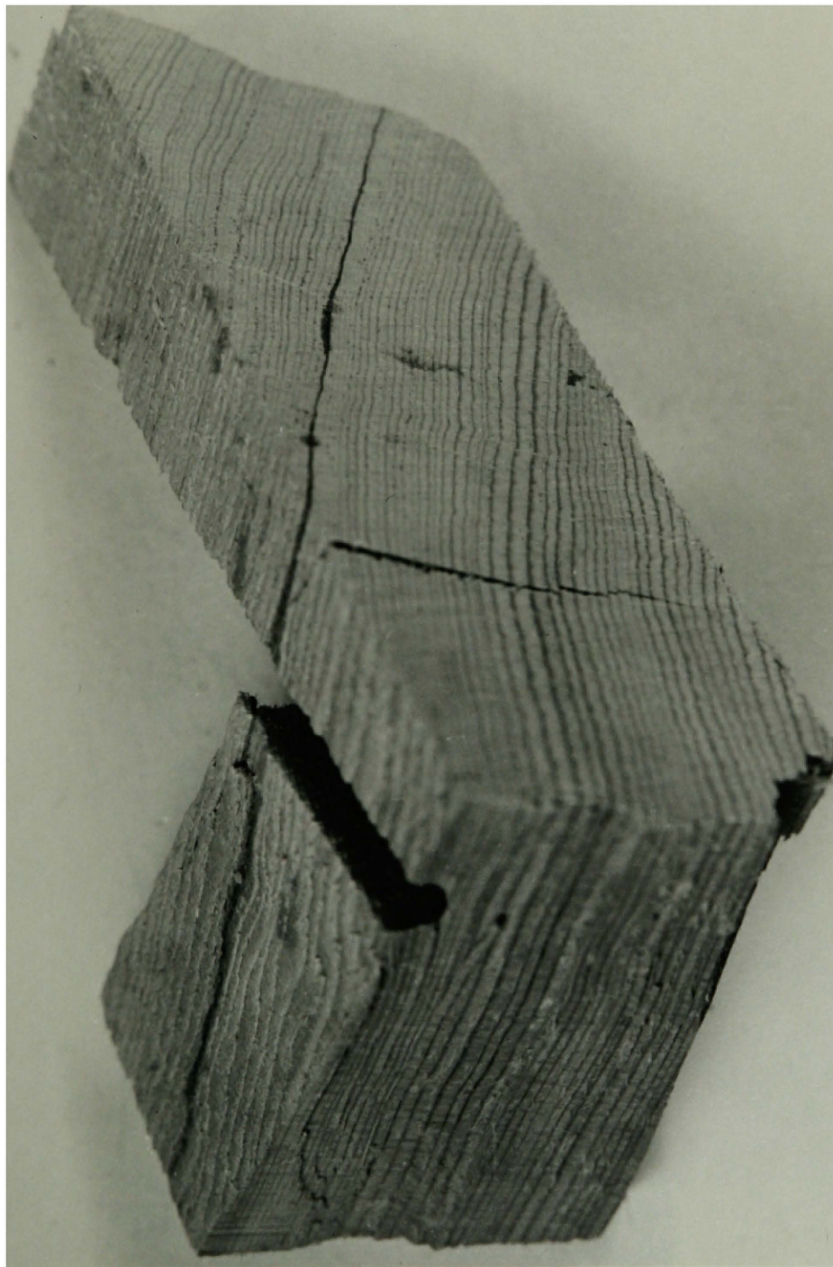
FIGURE 11. TYPICAL BLOCK SECTION FROM WHICH MICROSCOPIC EXAMINATION WAS MADE.
