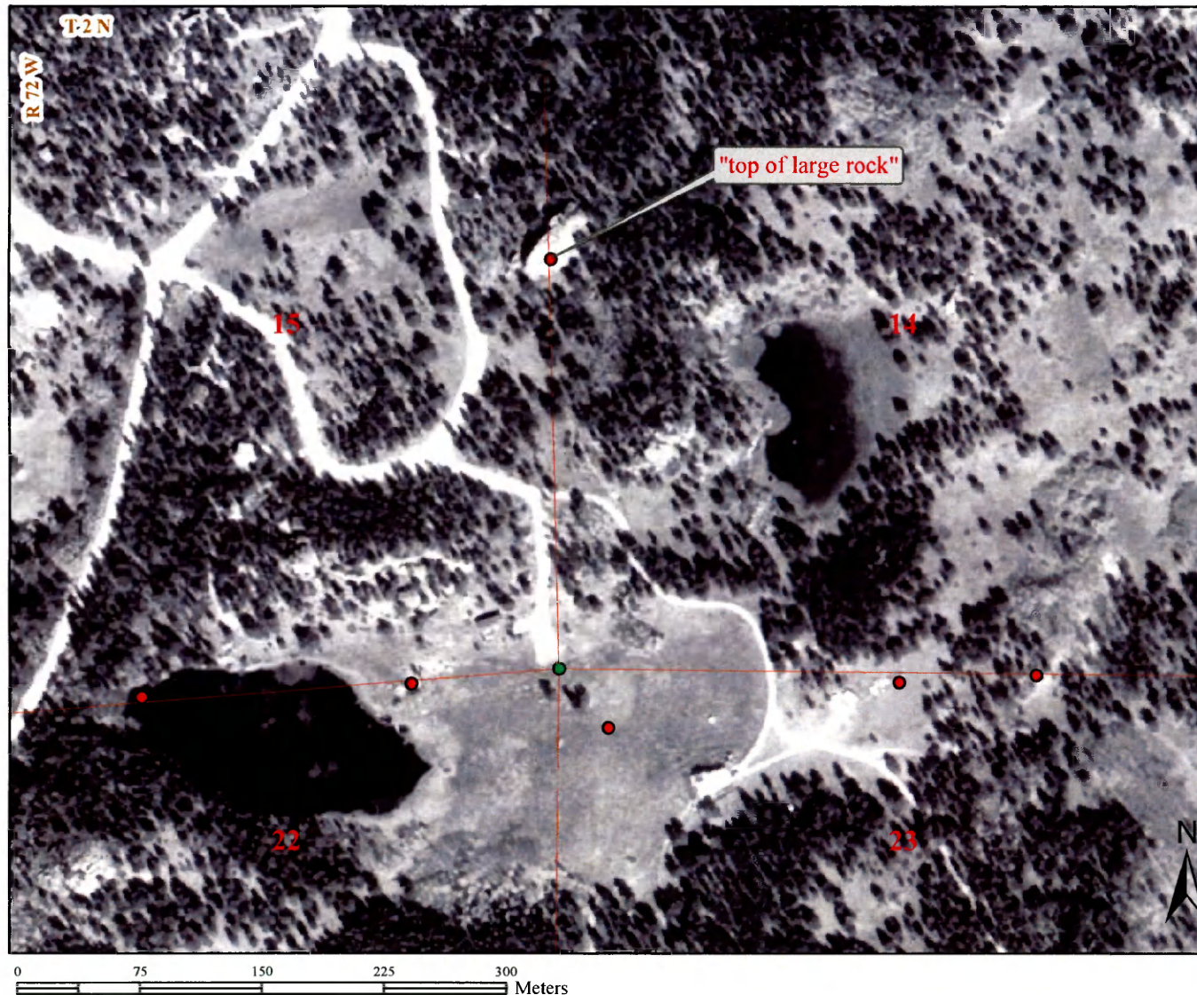
Figure 4.9 "Top of Large Rock." Note the accuracy in which the feature is recorded by the surveyor when plotted over the GCDB.
