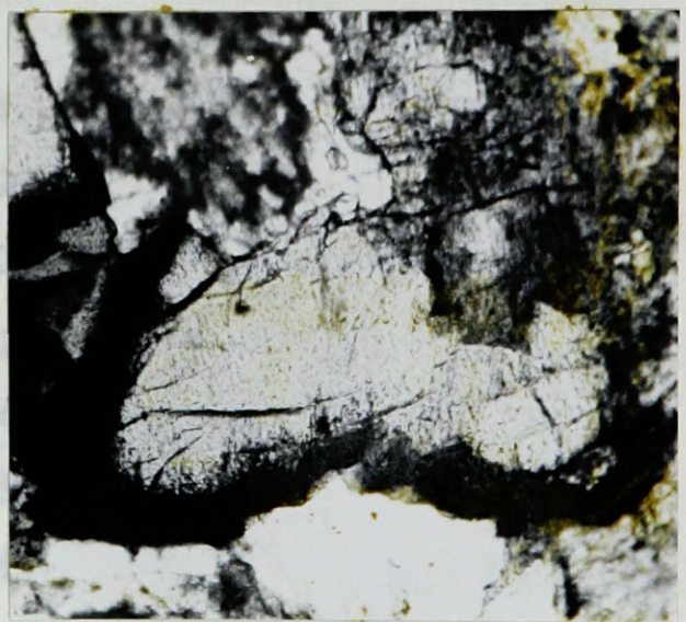
Figure 7. Photomicrograph of hornblende (dark) rimming pyroxene crystal (70X and plane light)
