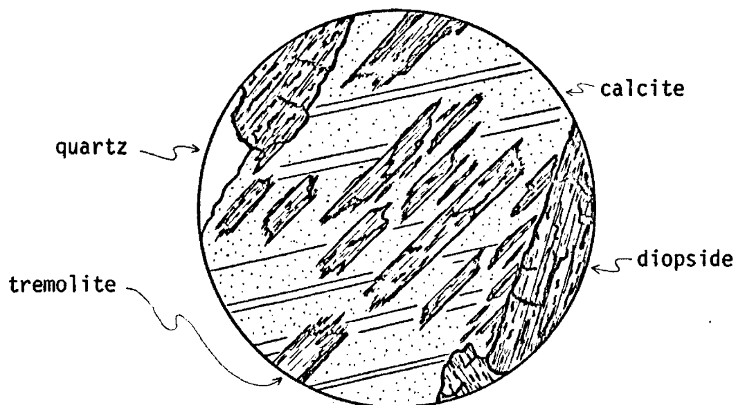
Fig. 3.15. (320X) Thin section sketch of a sample from the tremolite zone - diopside zone reaction boundary (reaction 5, p. 51). Diopside growing after actinolite as elongate prisms in presence of "clean" actinolite and calcite is seen under high power. Sample taken 1 mile northeast of northeast "tongue" of Skalkaho stock. Nature of this reaction and reaction boundary is discussed in text.
