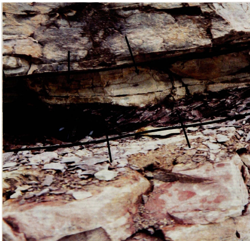
Figure 4b: Inclined cleavage to bedding, i.e. crenulation cleavage, in a K-bentonite from the McNamara Formation
