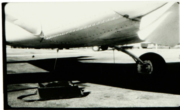
Fig. 7b.--Antennas installed on permanent attachments on Cessna 182 aircraft.
